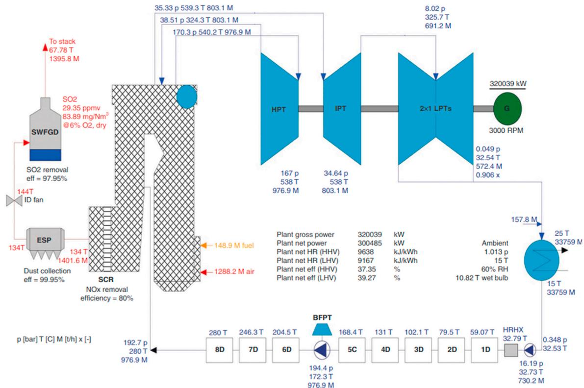
Fig. 14. Example of DT architecture for thermal power plant by Ref. [33].
