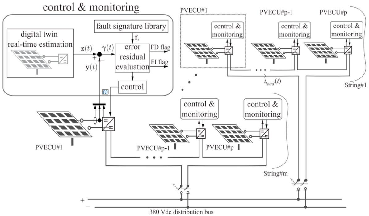
Fig. 7. Example DT Architecture in a PV system based on [40].
