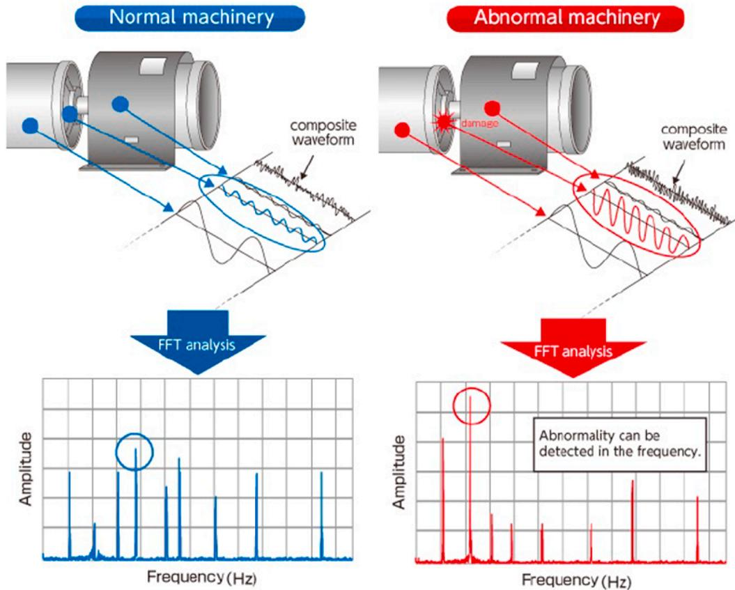
Fig. 13. Example of showing abnormalities using the FFT method based on [54].
