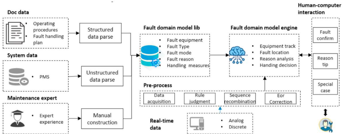
Fig. 10. Architecture of the hydropower plant fault diagnosis application [47].
