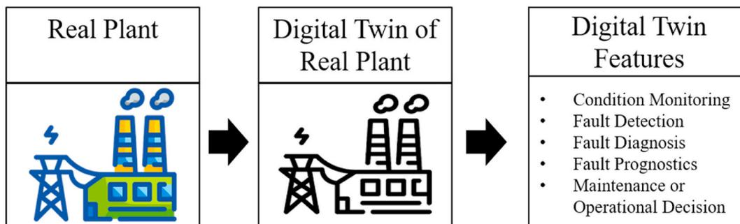
Fig. 15. Framework for digital twin in a nuclear power plant by Ref. [55].
