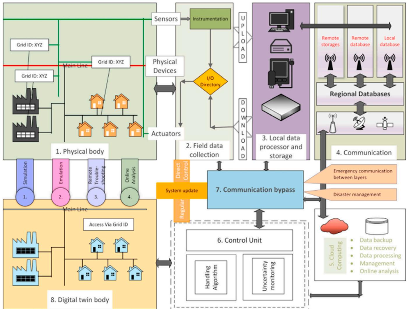
Fig. 16. Conceptual framework of electric digital twin grid [57].
