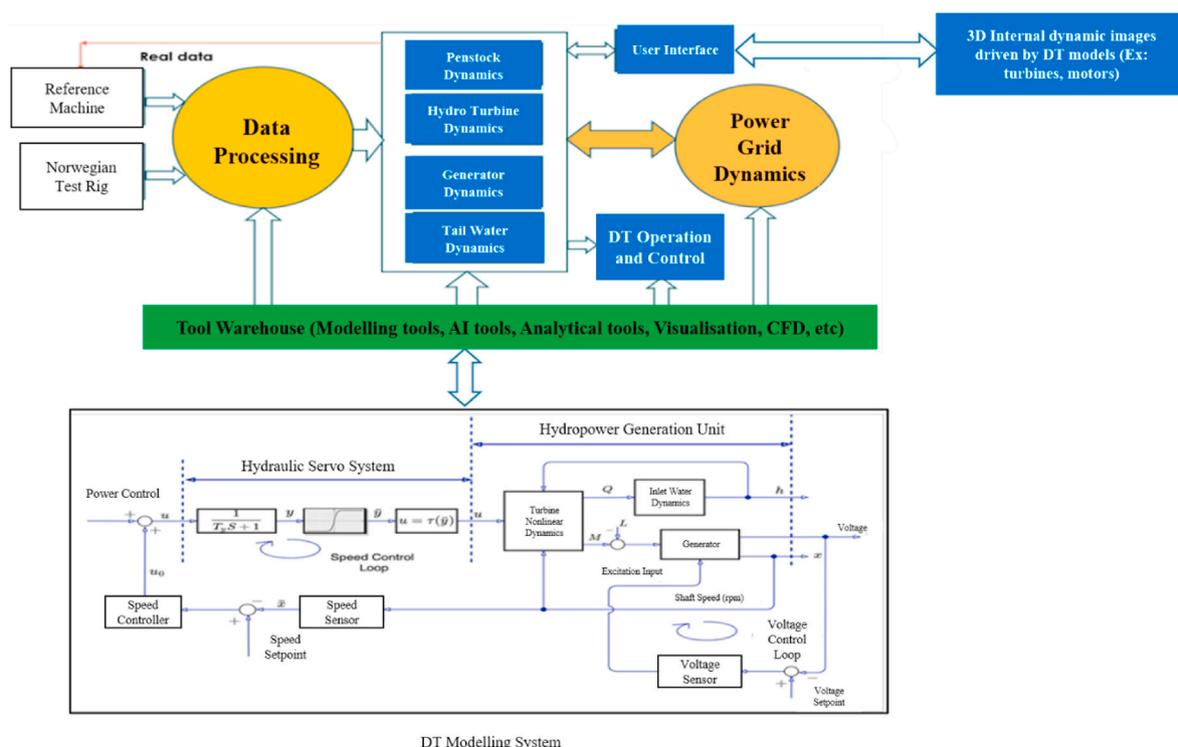
Fig. 9. Example DT architecture for hydropower plant based on [46].
