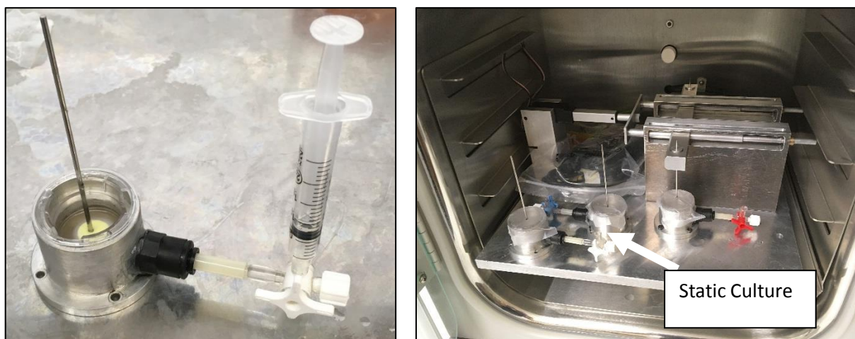
Figure 5.6: Images of pin machine during incubation and sampling of media from aluminium well. Skin models were placed in the aluminium wells and the skin pieced with a fixation wire. Notice the syringe attachment to the stopcock in order to sample media form below the transwell insert.
