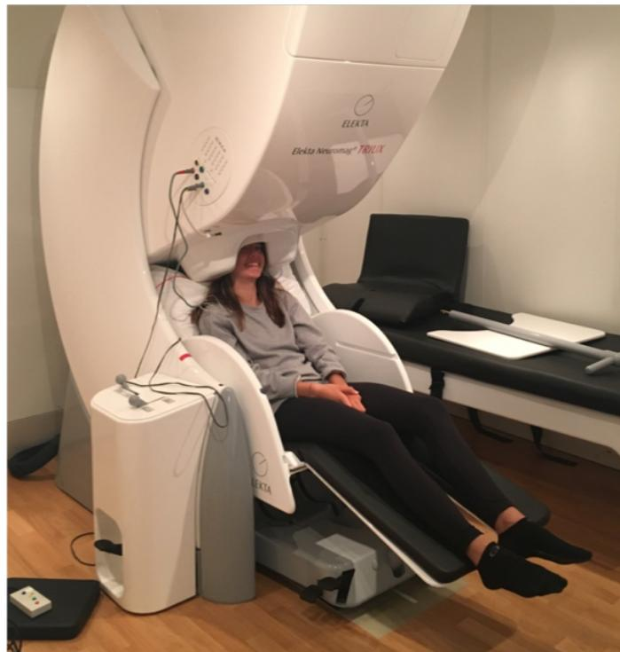
Fig. 2.3 Elekta Triux MEG machine in the magnetic shielded room (MSR) in the Aston Brain Centre, Aston University, Birmingham (UK).
