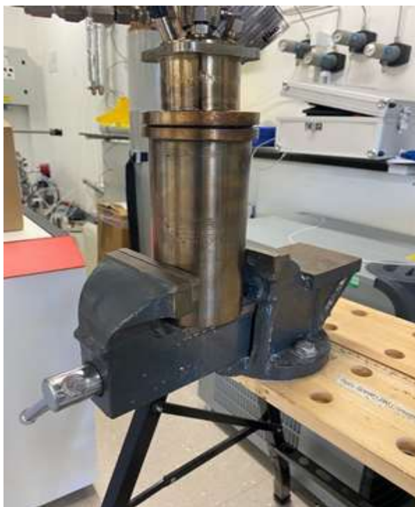
Figure 3.4: Arrangement for loading and unloading the 450 ml reactor using a laboratory vice
