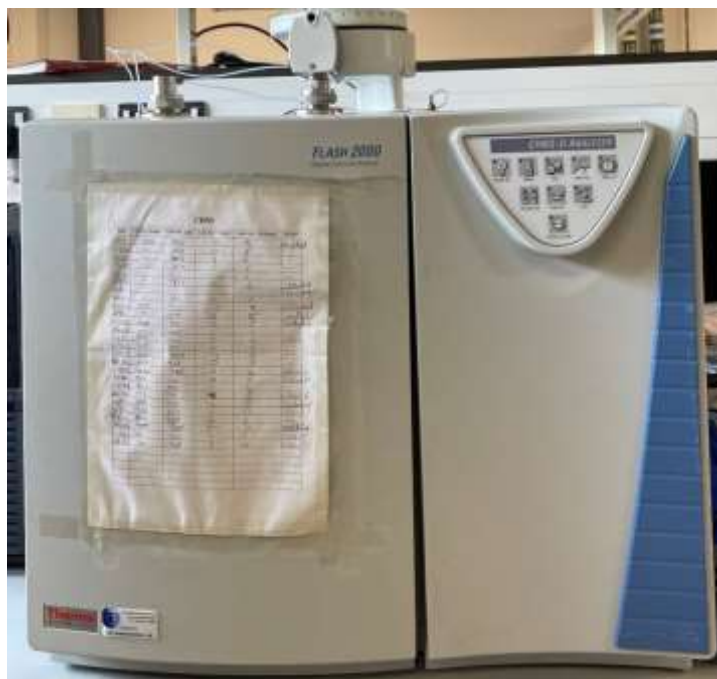
Figure 3.32: Photo of CHNS equipment used
