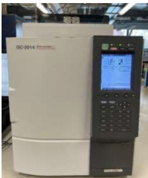
Figure 3.20: GC used for gas analysis
