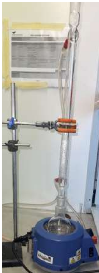
Figure 3.26: Photo of reflux set up used for esterification
