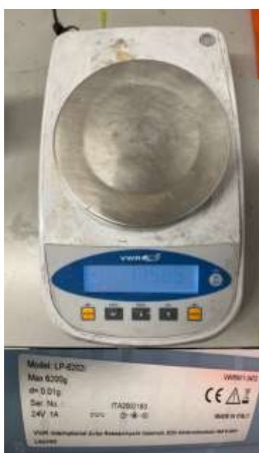
Figure 3.5: Photo of the main weighing balance used in this study
