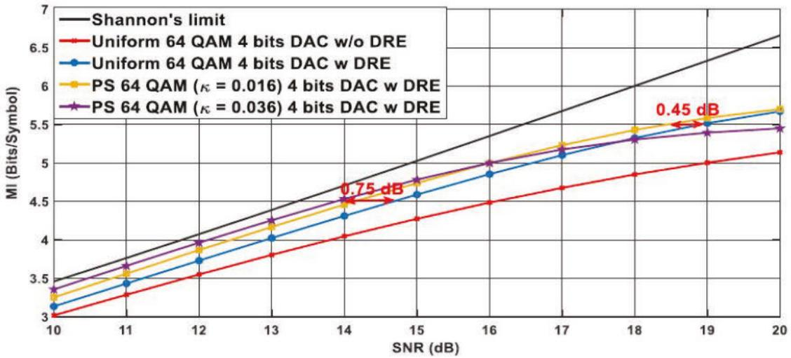
Fig. 5.7 Performance in terms of MI versus channel SNR for simulated 64-Gbd/64-QAM modulation in different scenarios with DRE compared to Shannon's limit (black) and uniform modulation w/o DRE (red)
