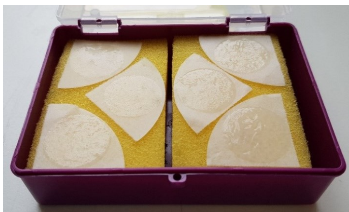
Figure 5.1 Experimental setup used in determination of water uptake and swelling index of the film manufactured.
