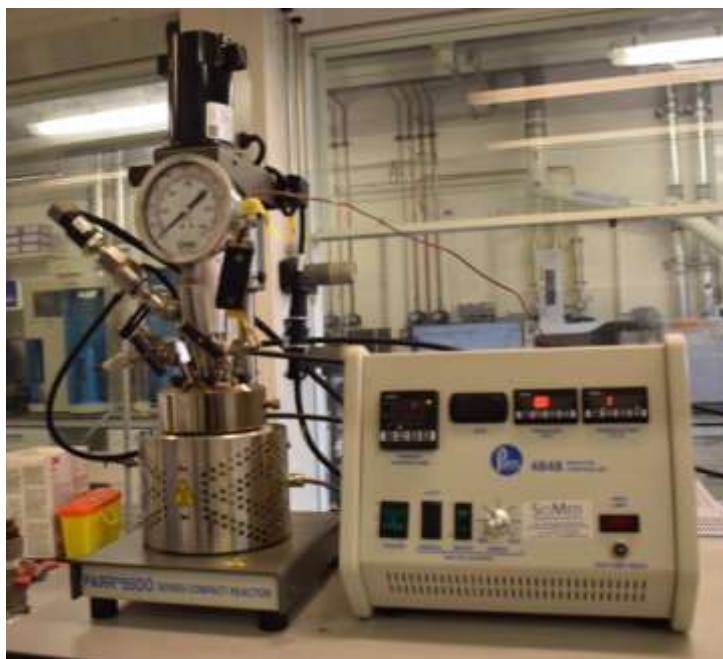
Figure 43. 300 ml stainless steel (T316) Parr® 5521 compact batch autoclave reactor (left) with Parr® 4848 reactor controller (right).
