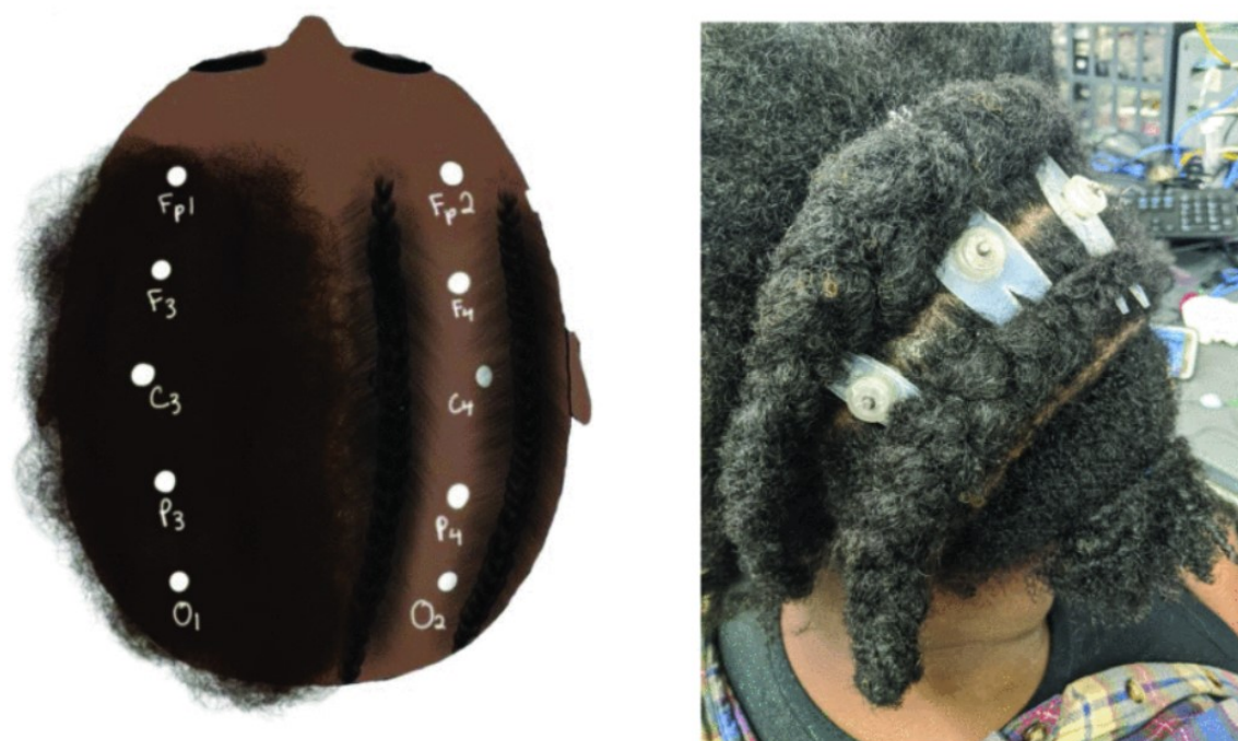
Figure 5.3: Image adapted from (Etienne et al., 2020). Shows the Sevo electrode and electrode-bearing hair clip placed between two canerows on Afro hair.
