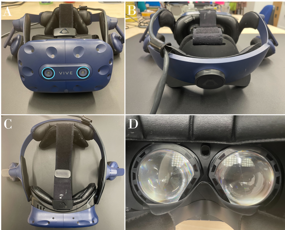
Figure 4.2: A combination of photographs taken of the HTC Vive Pro Eye. Photographs A-C show different angles of the headset with A presenting a front view. Picture labeled B shows the head support at the back with the black circle to adjust the headset in length. C is an overhead view with the adjustable strap to help keep the display in position and alleviate some of the weight from the face. Lastly, image D, shows the black dashes around the lenses, which correspond to the eye-tracker.
