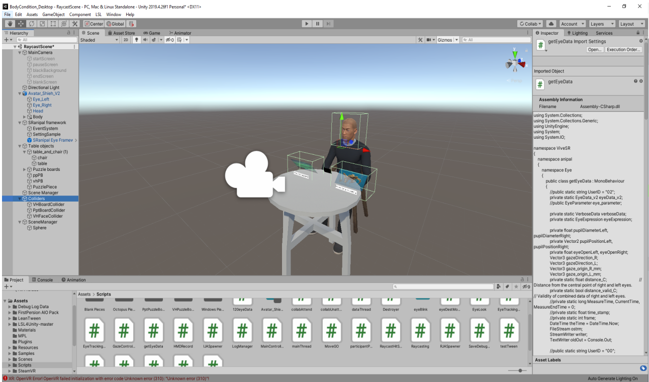
Figure 4.5: A still image of the colliders that were used as regions of interest for the participants’ eye-tracking data. They have been made visible in the virtual environment (highlighted in green) for visualising purposes.
