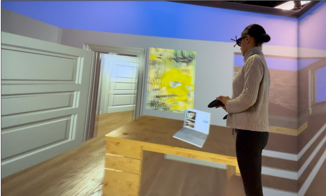
Figure 5.1: A picture demonstrating a user traversing a CAVE environment whilst wearing stereoscopic 3D glasses
