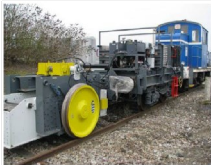
Figure 2.9: On-site measurement using the Portancemètre in Rouen, France (Do, 2020)
