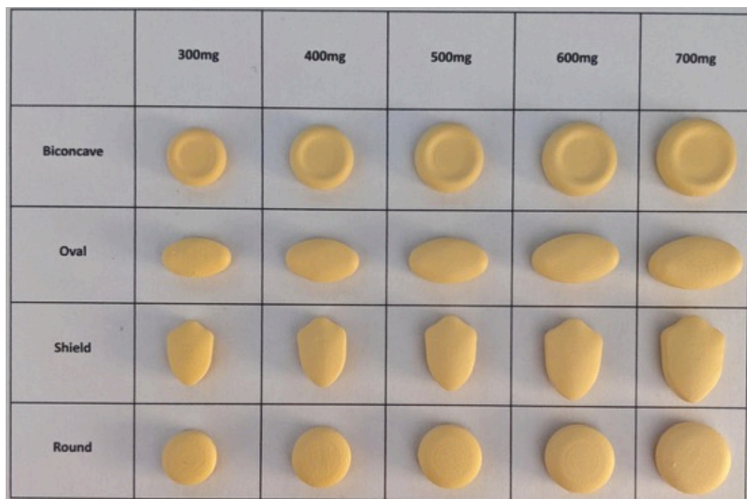
Figure 6.3 3D printed tablet models produced at Colorcon, Dartford
