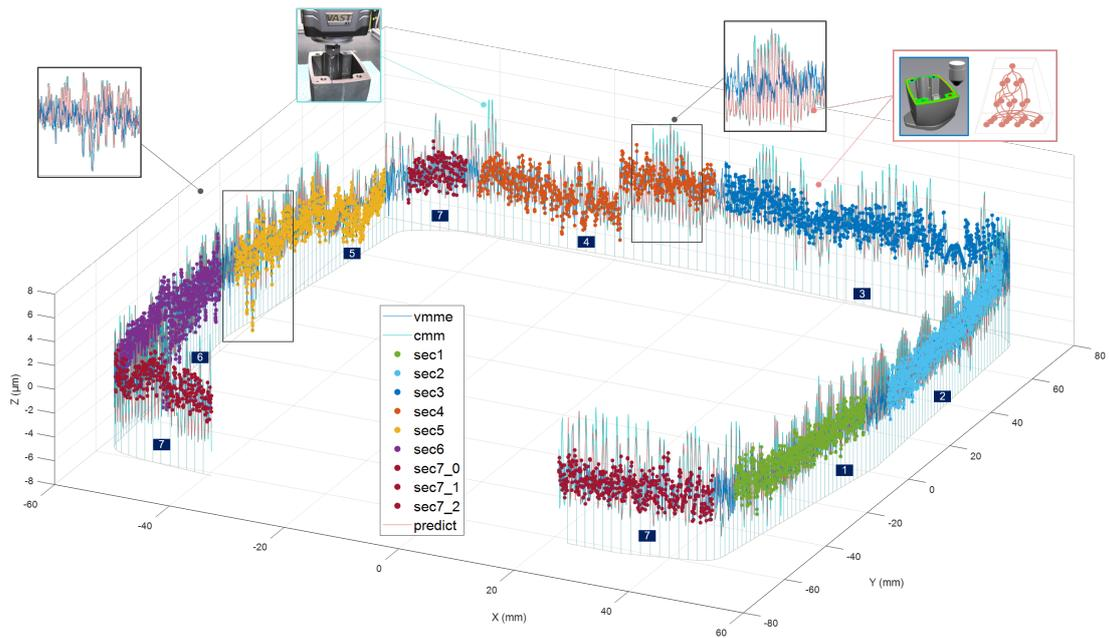
Figure 12: DT results with UQ. Measured and modeled flatness of the selected surface.
