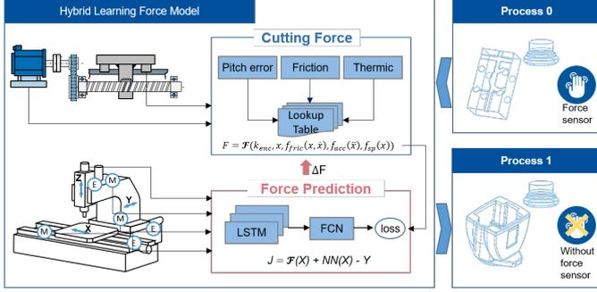
Figure 11: Transfer of the pre-trained force model into the hybrid model chain.
