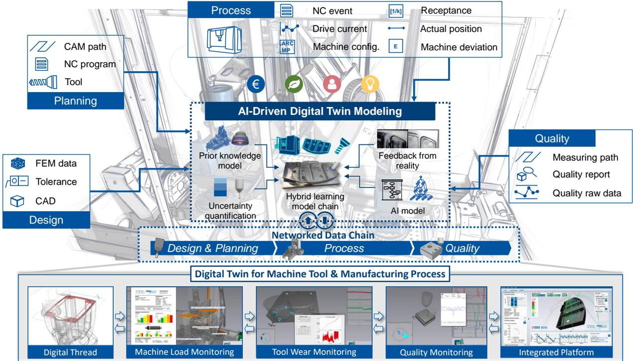
Figure 2: The motivation and objective of AI-driven digital process twins, modified from [5]. ©WZL-RWTH Aachen.
