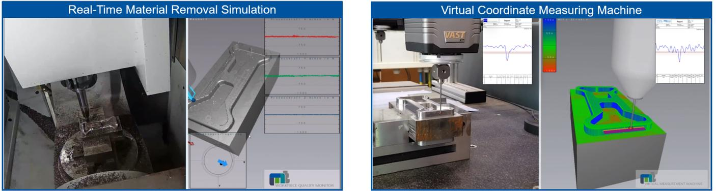
Figure 1: Process-parallel prediction of workpiece quality via a digital process twin at the EMO Hannover 2019. Deployed machine: Chiron FZ 12. ©WZL-RWTH Aachen, MT Analytics GmbH.
