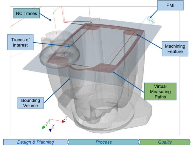
Figure 8: The feature-based digital thread of contextualized metadata sources across the manufacturing procedure: design, planning, NC process, and quality inspection.
