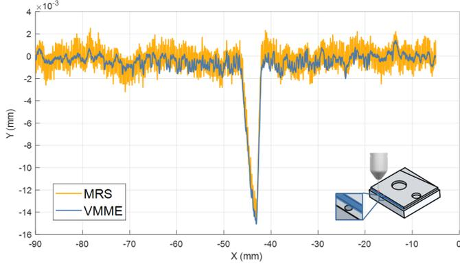
Figure 7: Comparison of estimated workpiece quality using the MRS and VMME.
