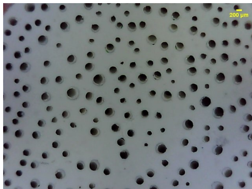
Figure 6.9 Digital microscope image of the bottom-surface of the NMP-PMMA-56 membrane
