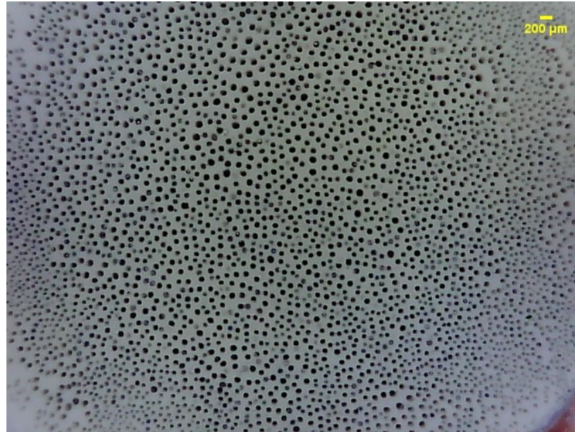
Figure 6.7 Digital microscope image of the top-surface of the sanded NMP-PMMA-56 membrane
