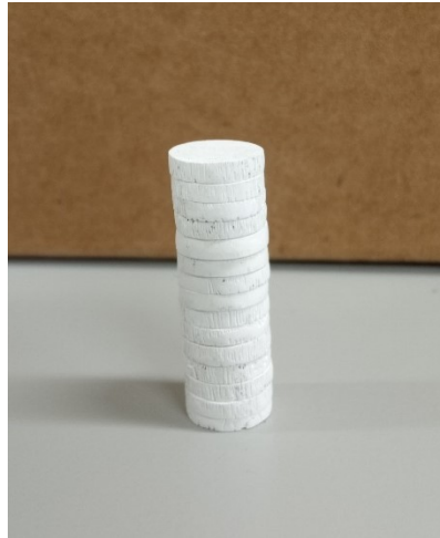
Figure 3.6 Stacked membranes outside of the reactor tube
