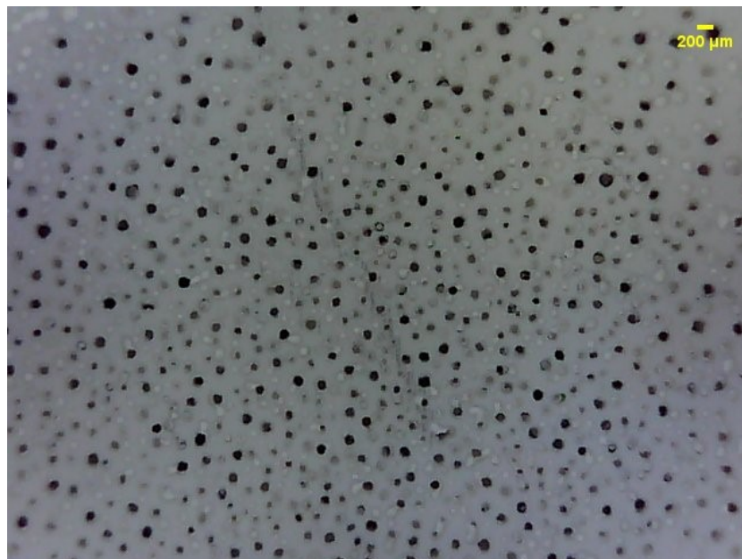
Figure 6.8 Digital microscope image of the top-surface of the sanded NMP-PMMA-60 membrane
