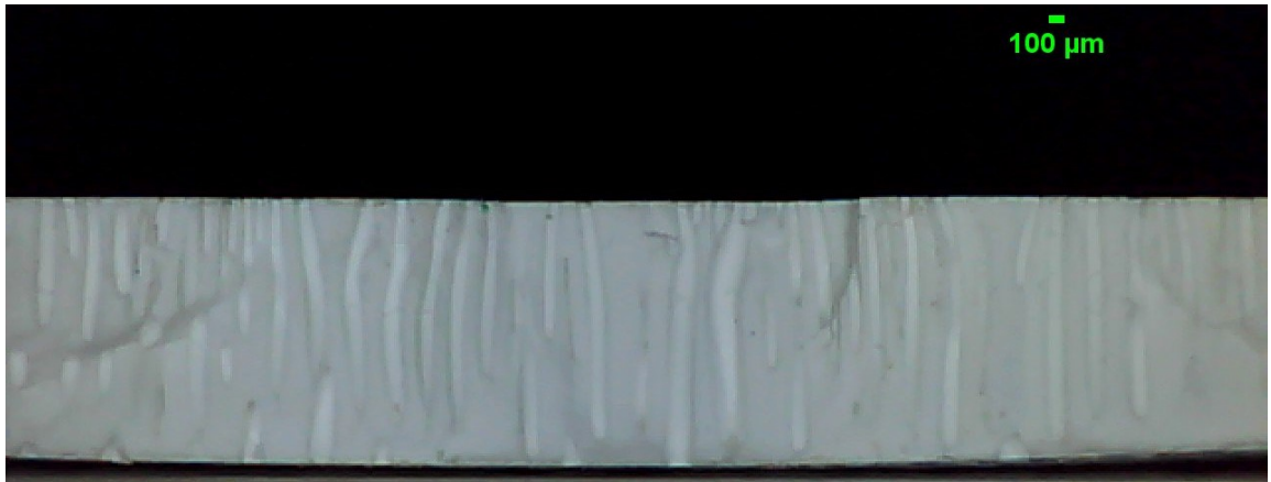
Figure 6.5 Digital microscope image of the cross-section of the NMP-PMMA-56 membrane with top and bottom skin-layers removed
