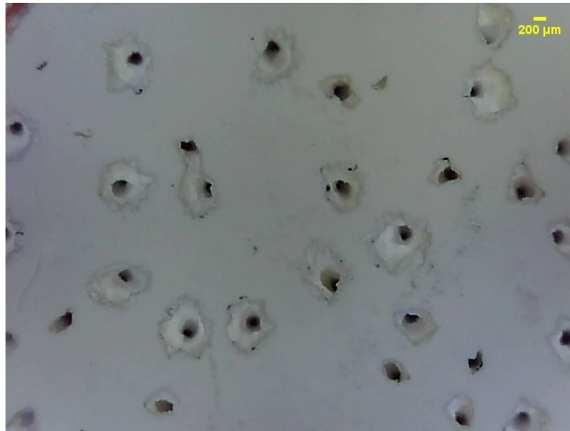
Figure 6.10 Digital microscope image of the bottom-surface of the NMP-PMMA-60 membrane
