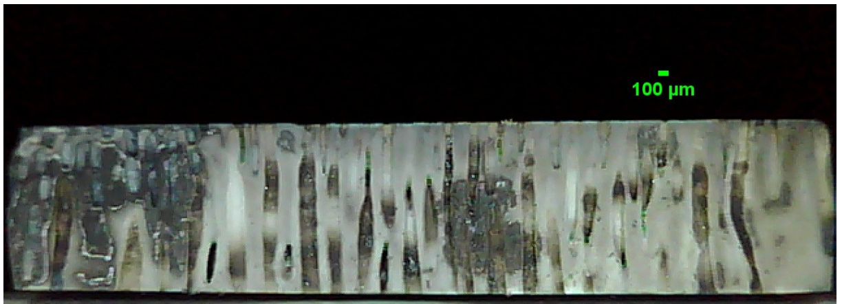
Figure 6.11 Digital microscope image of the NMP-PMMA-56 spent membrane cross-section
