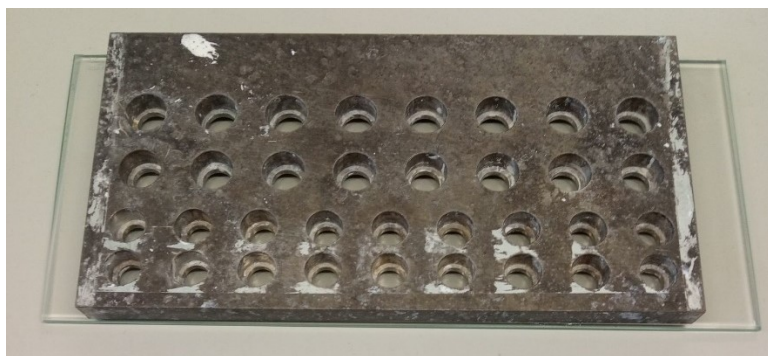
Figure 3.12 Aluminium mould and glass plate
