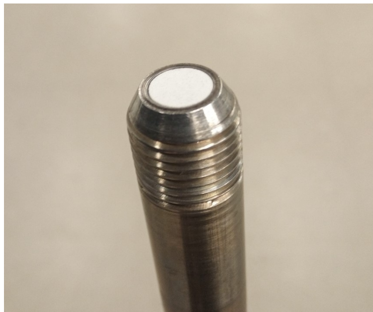
Figure 3.7 Membrane inside the entrance to the reactor
