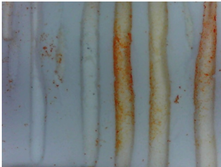
Figure 6.15 Cross-section of an NMP-PMMA-56 membrane after deposition with Co-MOF-74
