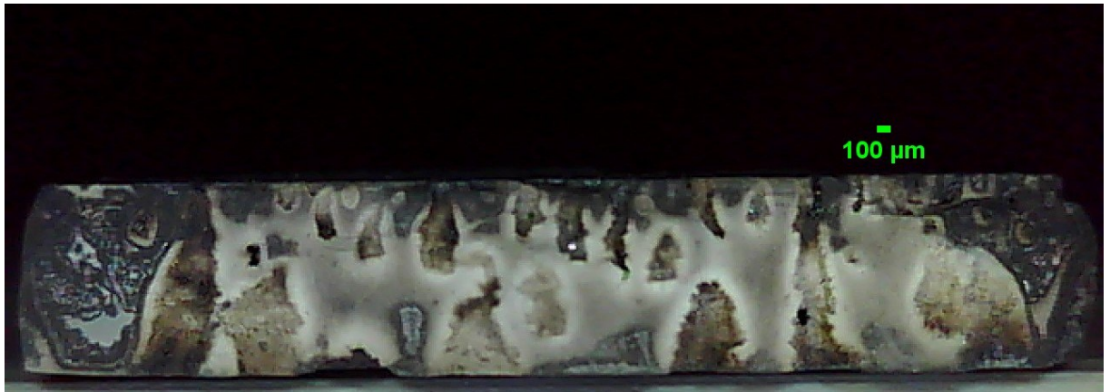
Figure 6.12 Digital microscope image of the NMP-PMMA-60 spent membrane cross-section
