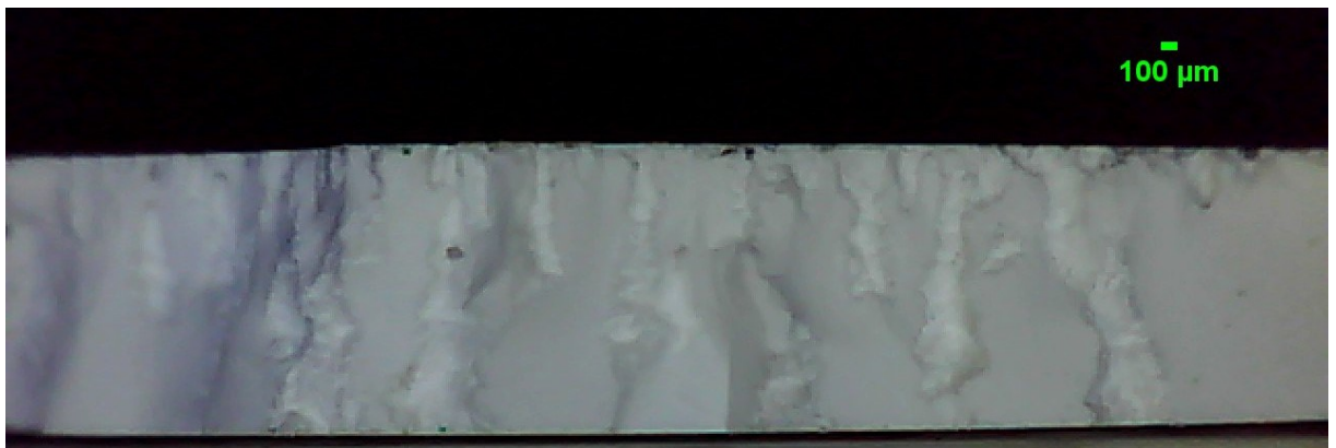
Figure 6.6 Digital microscope image of the cross-section of the NMP-PMMA-60 membrane with top and bottom skin-layers removed
