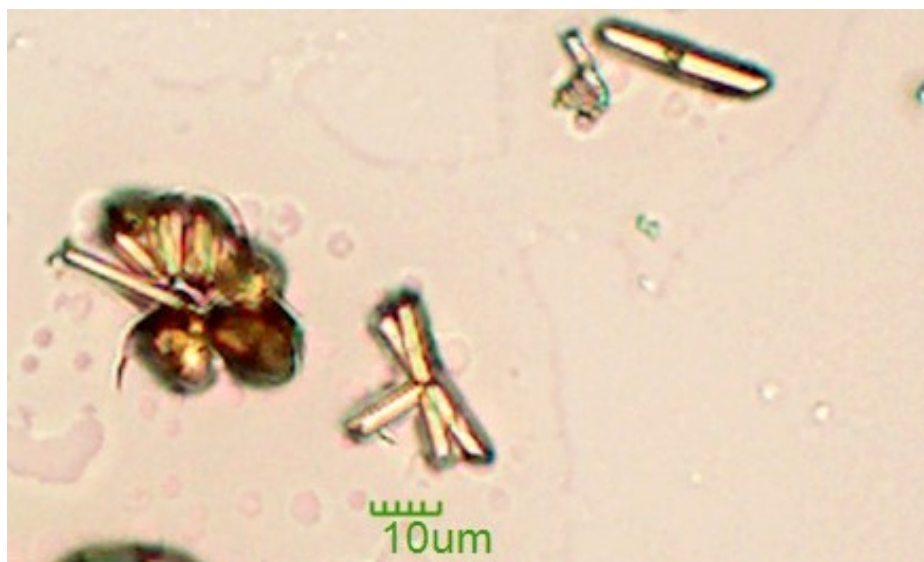
Figure 4.4 Microscope image of Co-MOF-74 crystals
