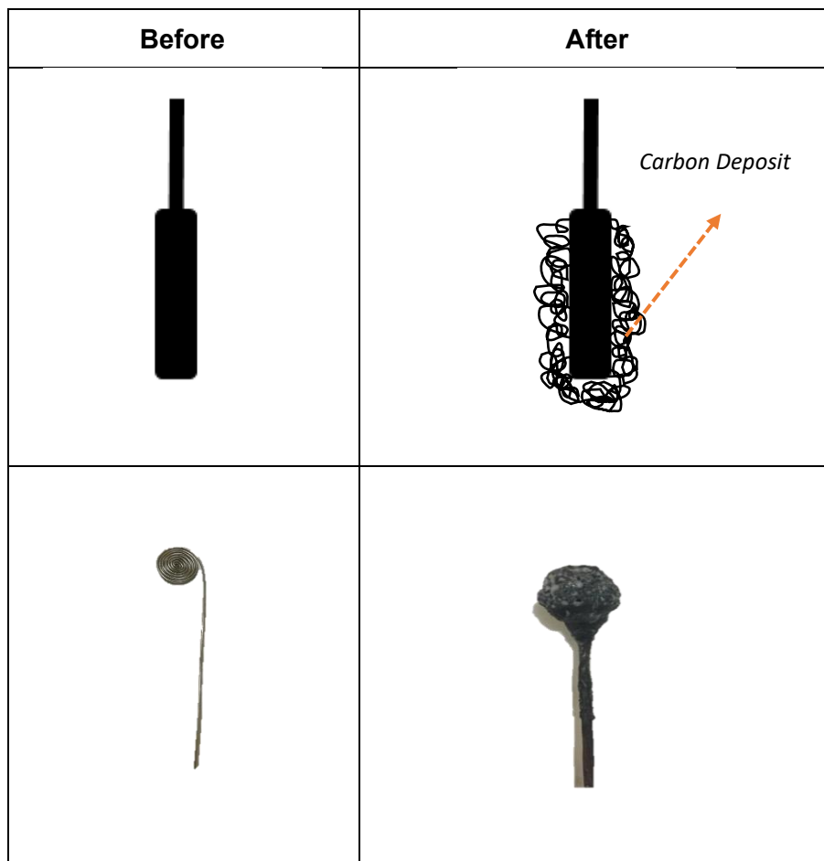
Figure 52 Electrode profile before and after the Electrodeposition process
