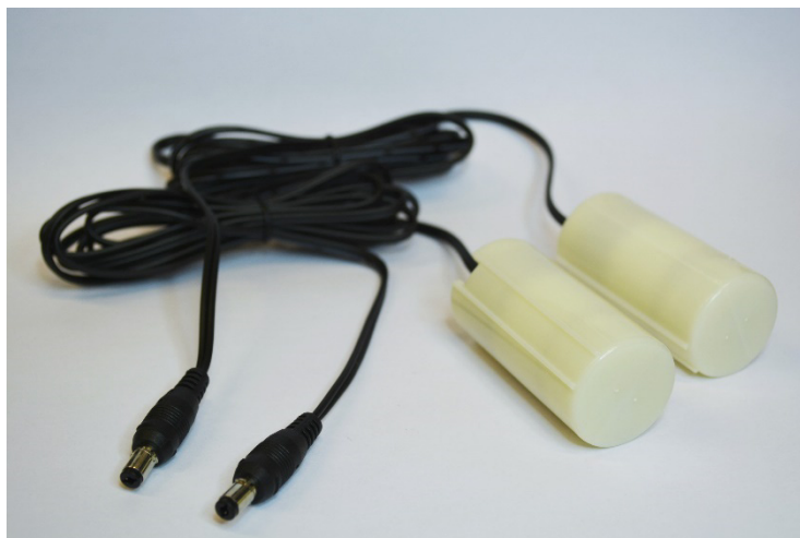
Figure 3.1. Custom-made vibrators used to administer the proprioceptive stimulation. Each plastic cylinder contains a DC motor and an eccentric rotating mass
