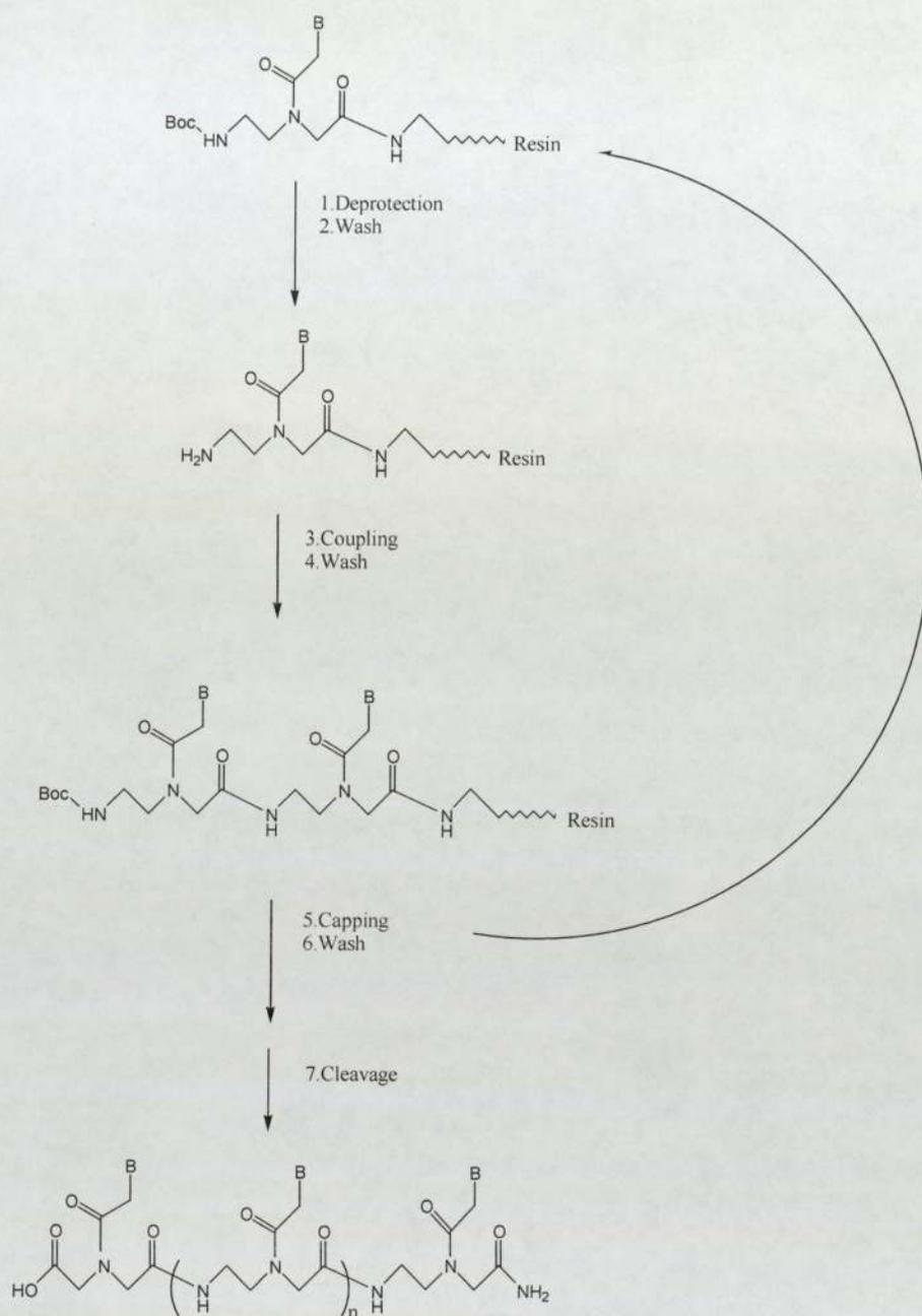
Figure 10. Schematic representation of the solid phase PNA synthesis
