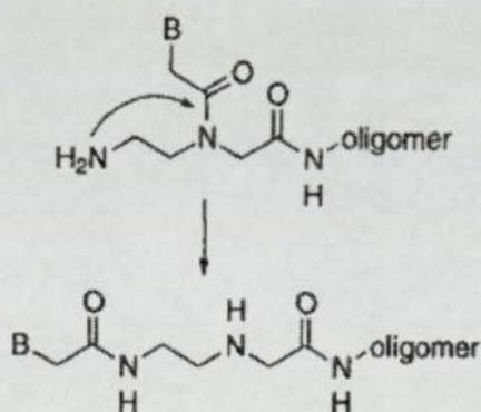
Figure 4. The N-acyl transfer reaction
