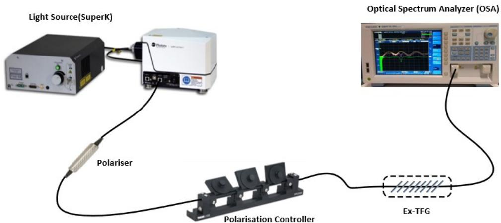
Figure 3. 27 Experimental setup for measuring transmission spectra of Ex-TFG.
