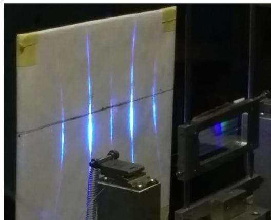
*Figure 3. 2 Diffraction pattern when the SMF-28 fibre is placed in front of the phase mask for grating inscription.*
