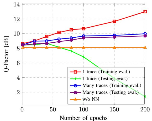
Fig. 9: Q-factor versus training epochs for the experiment with 16-QAM  $5 \times 50$  km SSMF, 34.4 GBd, 6 dBm power, using the biLSTM equalizer. These curves refer to the training and testing performance of the NN when using one trace or when using multiple traces (our solution is described in the main text) for training.
