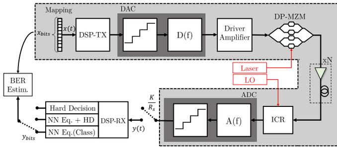
Fig. 1: Experimental setup used to analyze the performance of NN equalizers;  $D(f)$  is the DAC electrical transfer function,  $A(f)$  is the ADC electrical transfer function, and  $x(t)$  and  $y(t)$  are the transmitted/received time sequences of symbols, respectively. The input of the NN is the soft output of the regular DSP just before the decision module.
