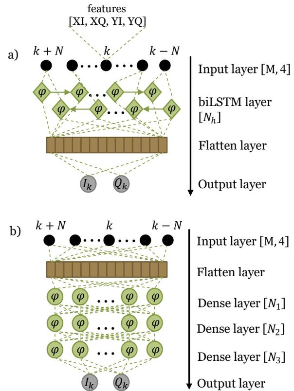
Fig. 2: The schematics of different NN architectures considered in our paper: a) biLSTM equalizer with  $N_h$  hidden units and b) MLP equalizer having three hidden layers, with  $N_1$ ,  $N_2$ , and  $N_3$  neurons in each consecutive layer, respectively. The input has a memory equal to  $M = 2N + 1$  and 4 features representing the real (I) and imaginary (Q) parts of both X and Y polarizations. The function  $\varphi$  represents the activation function which in our case is the “tanh”.
