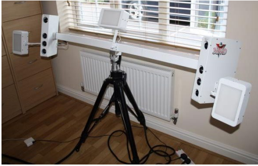
Figure 2.1a. The 3dMDFace™ measurement system adapted for portability by attaching to a regular camera tripod and altering the design of the horizontal camera brace bar.
