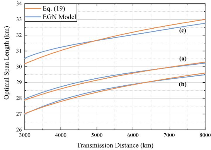
**Fig. 4.** The optimal span length versus the transmission distance. (a) 64 GBaud 71 channels at -2 dBm per channel, EDFA noise figure is 6 dB; (b) 32 GBaud 141 channels at -5 dBm per channel, EDFA noise figure is 6 dB; (c) 64 GBaud 71 channels at -2 dBm per channel, EDFA noise figure is 4.5 dB
