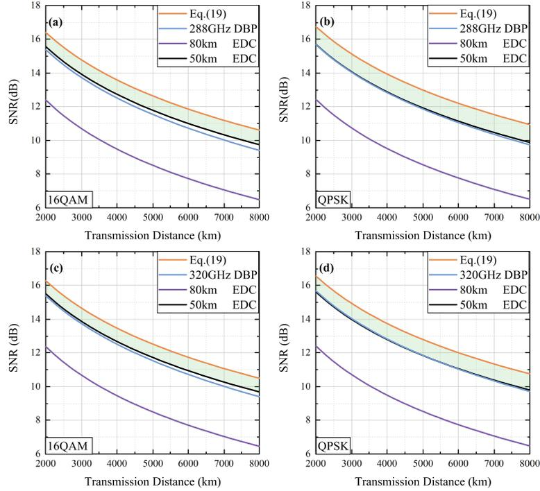
**Fig. 7.** The SNR at different transmission schemes. Orange lines: the theoretical optimal span length calculated by Eq. (19). Blue lines: 80 km per span using MC-DBP. Purple lines: 80 km per span EDC only. Dark lines: 50 km per span EDC only. (a) and (b) 32 GBaud 61 channels at optimal launched power; (c) and (d) 64 GBaud 33 channels at optimal launched power.
