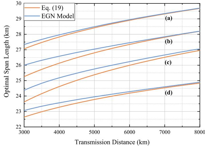
**Fig. 3.** The optimal span length v.s. transmission distance. (a) 128 GBaud 15 channels at 1 dBm per channel; (b) 64 GBaud 33 channels at -2 dBm per channel; (c) 32 GBaud 61 channels at -5 dBm per channel; (d) 48 GBaud 51 channels at -4 dBm per channel. EDFA noise figure is 6 dB in all curves.
