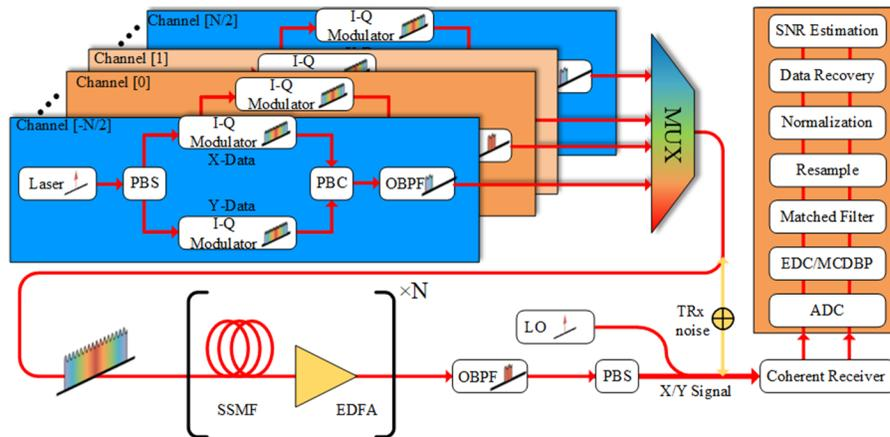
**Fig. 1.** Schematic of the dual-polarization multi-channel Nyquist-spaced optical fiber communication system. PBS: polarization beam splitter, PBC: polarization beam combiner, LO: local oscillator, ADC: analogue-to-digital convertor, OBPF: optical band-pass filter.
