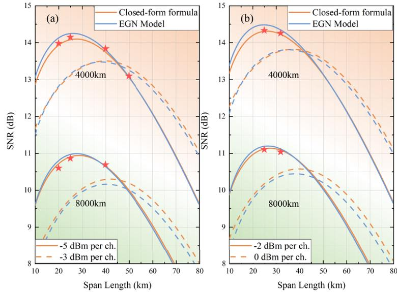
**Fig. 2.** The accuracy of closed-form formula in Eq. (12), compared to the EGN model. (a) 61 channels and 32 GBaud per channel. (b) 33 channels and 64 GBaud per channel. Red dots are simulation results.
