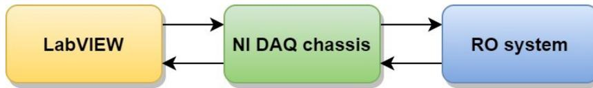
**Fig. 3.19.** Data-acquisition and control system structure.
