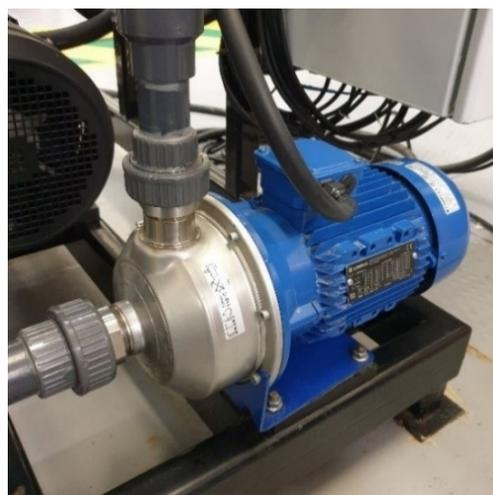
**Fig. 3.7.** Low-pressure pump.
