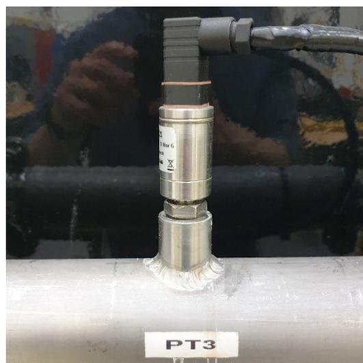
**Fig. 3.13.** Pressure transmitter.
