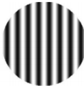
Figure 4.11: DMD interferogram in an ideal case.
