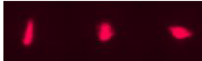
Figure 4.14: Beam spots taken from the same radial distance from the DMD while the focal length is varied [62].
