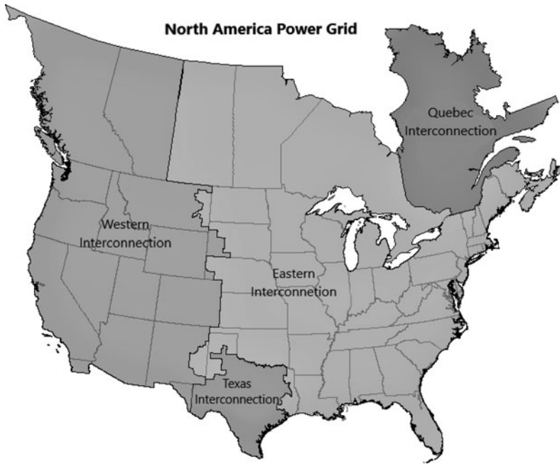
Figure 2. Map of North American energy interconnections. (Source: Image adapted, with permission, from the Western Electricity Coordinating Council [WECC], https://www.wecc.org/epubs/StateOfTheInterconnection/Pages/The-Bulk-Power-System.aspx .)
