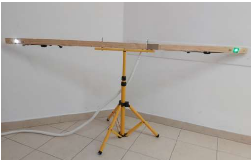
Figure 2.1. A photograph of the central (white LED) and eccentric (green LED) fixation targets, as viewed in the experimental setup.
