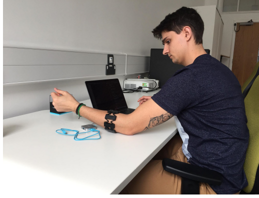
Figure 5.33: Data collection from a male subject via the Myo armband on their left arm.
