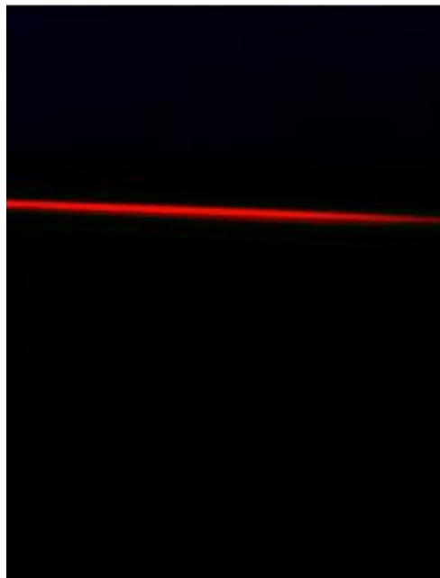
Figure 8. Image captured on camera of extended focal spot from an LED at 617nm
