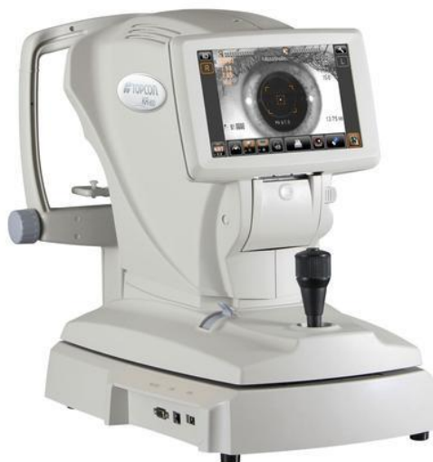
Figure 3.9 Topcon KR800 auto kerato-refractometer (Topcon Medical systems Incorporated, Fukuoka, Japan) (193), used to measure the ocular refraction.
