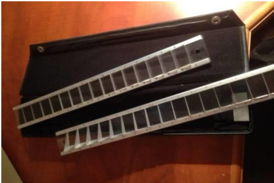
Figure 1.6 Photograph of the Clement Clarke Prism Bars used for measuring ocular alignment and all fusion measurements. The prism bar increments (steps) are 1 - 2 - 4 - 6 - 8 - 10 - 12 - 14 - 16 - 18 - 20 - 25 - 30 - 35 - 40 - 45^{\Delta} . ( ^{\Delta} denoting prism dioptres).
