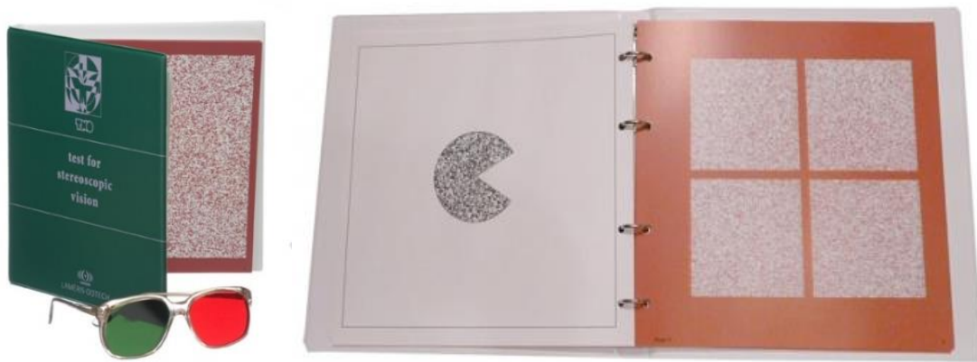
Figure 1.8 Photograph on left shows the TNO stereotest book and accompanying red/green glasses (Lameris Ootech BV, Nieuwegein, Netherlands). The right eye views the stereotest through the green filter, and the image appears green, while the left eye views the stereotest through the red filter, and image appears red. The two images should then be fused to see the image in 3-D, and hence measure stereoacuity. Photograph on right shows the pages inside the book demonstrating “cake with missing piece” or “PAC-MAN”, and the stereotest page where the patient must locate the “PAC-MAN” in each of the four squares.
