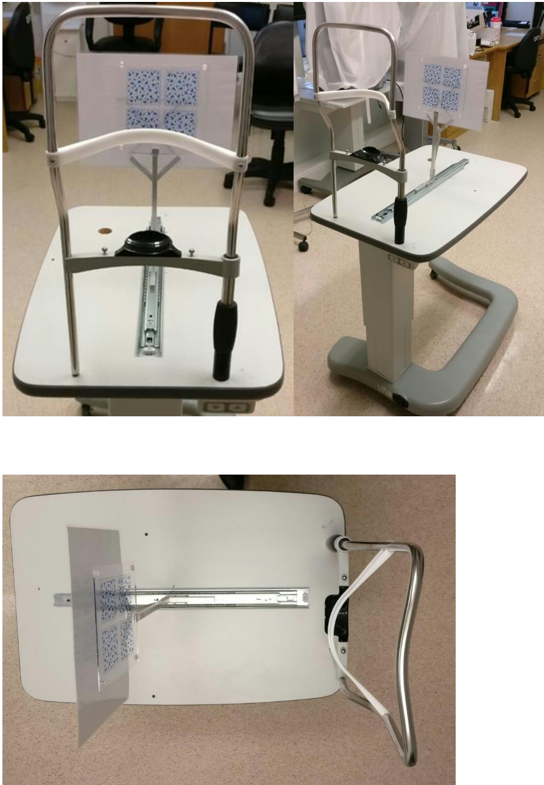
Figure 3.6 The researcher's proprietary designed gantry system for holding the Frisby stereotest plates, the design aim was to ensure accurate measurement of the distance from participant to plate.
