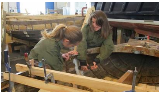
Fig. 5: Roving a steam-bent rib.
