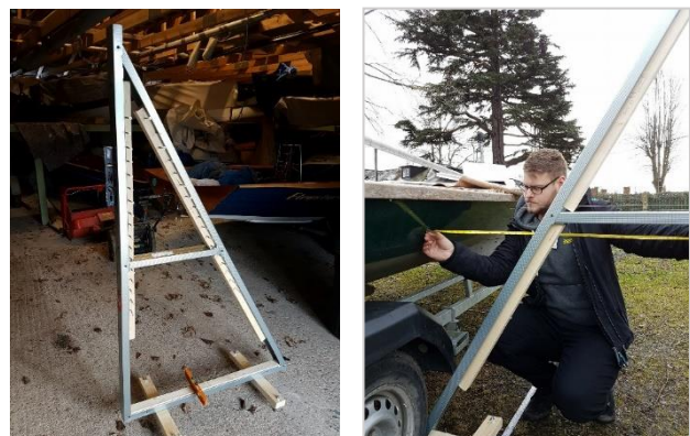
Figure 9: Rig used to take offsets from hull
