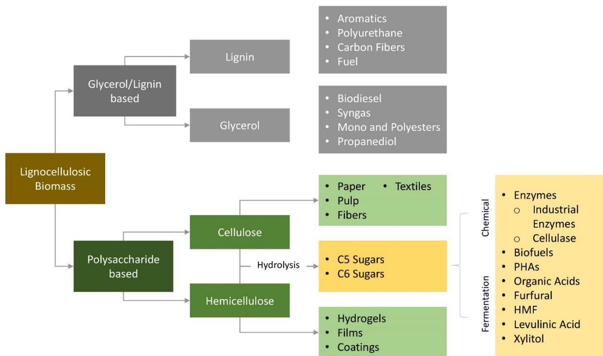
**Figure 1.** Valorization of lignocellulosic biomass into bioproducts and chemicals
