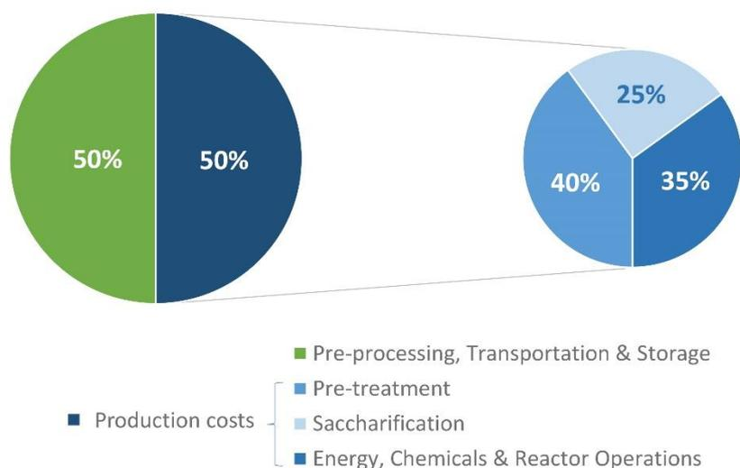
Figure 5. Cost breakdown of the steps involved in lignocellulosic biomass conversion
