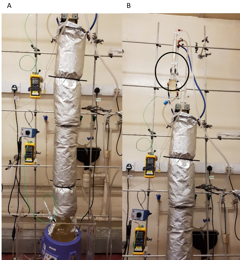
Figure 11.2. Distillation column in its typical setup, heat is applied to the 3 necked flask via the mantle it is placed in (2a). 2 temperature probes set up, one typically measuring the base temperature and the other measuring the temperature at the top of the column. For the first pass of the reaction, which involves an esterification, the overheads are fitted with a D&S (2b, circled) to collect water from the esterification reaction. (Overheads here refer to the glass equipment fitted on top the column which differs depending on the type of reaction being carried out e.g. D&S.)
