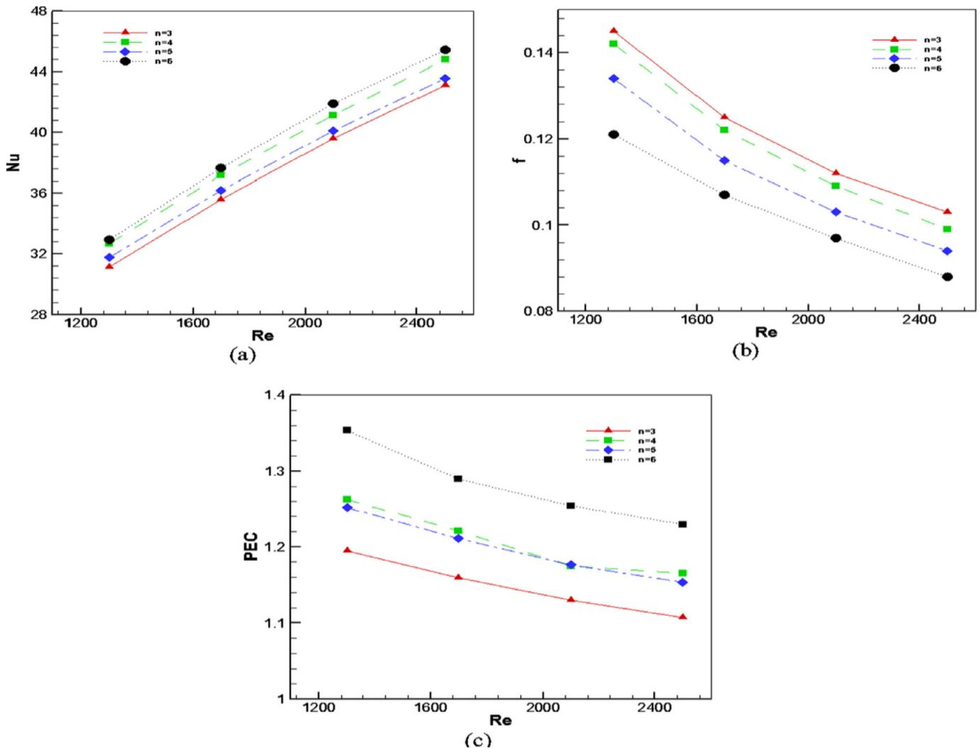
Fig. 8. Characteristics of flow in a helical coil subject to the number of lobes (a)  $Nu$  number (b) Friction factor, and (c) Performance evaluation criteria PEC, with permission from Elsevier [185].
