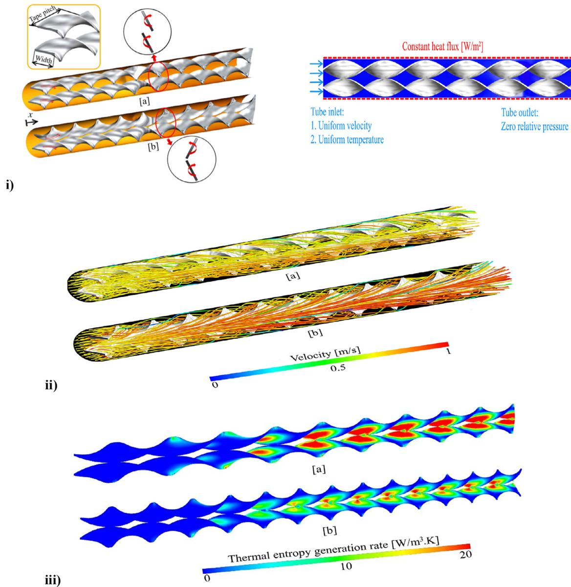
**Fig. 10.** Double twisted (i) geometry, (ii) flow pathlines, (iii) thermal entropy for (a) Co-twisted tapes (CoTs) (b) Counter twisted tapes (CTs), adapted with permission from Elsevier [188].
