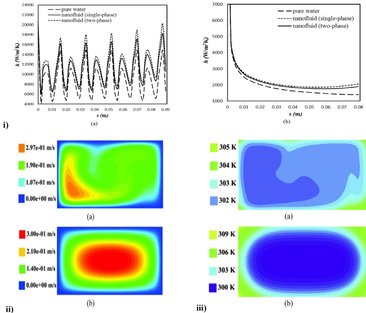
**Fig. 14.** (i) Convective heat transfer coefficient, (ii) Velocity counters, and (iii) Temperature counters for (a) C-shaped, and (b) Straight channel, adapted with permission from Elsevier [191].
