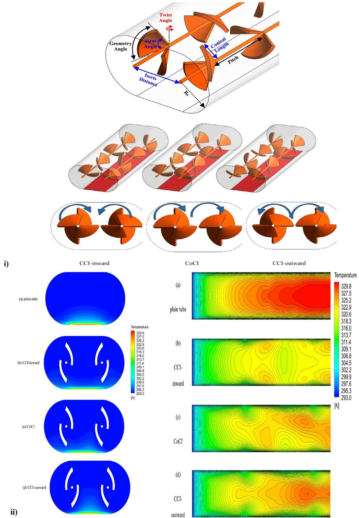
Fig. 12. (i) Geometrical structure of conical inserts, (ii) temperature contours, adapted with permission from Elsevier [189].
