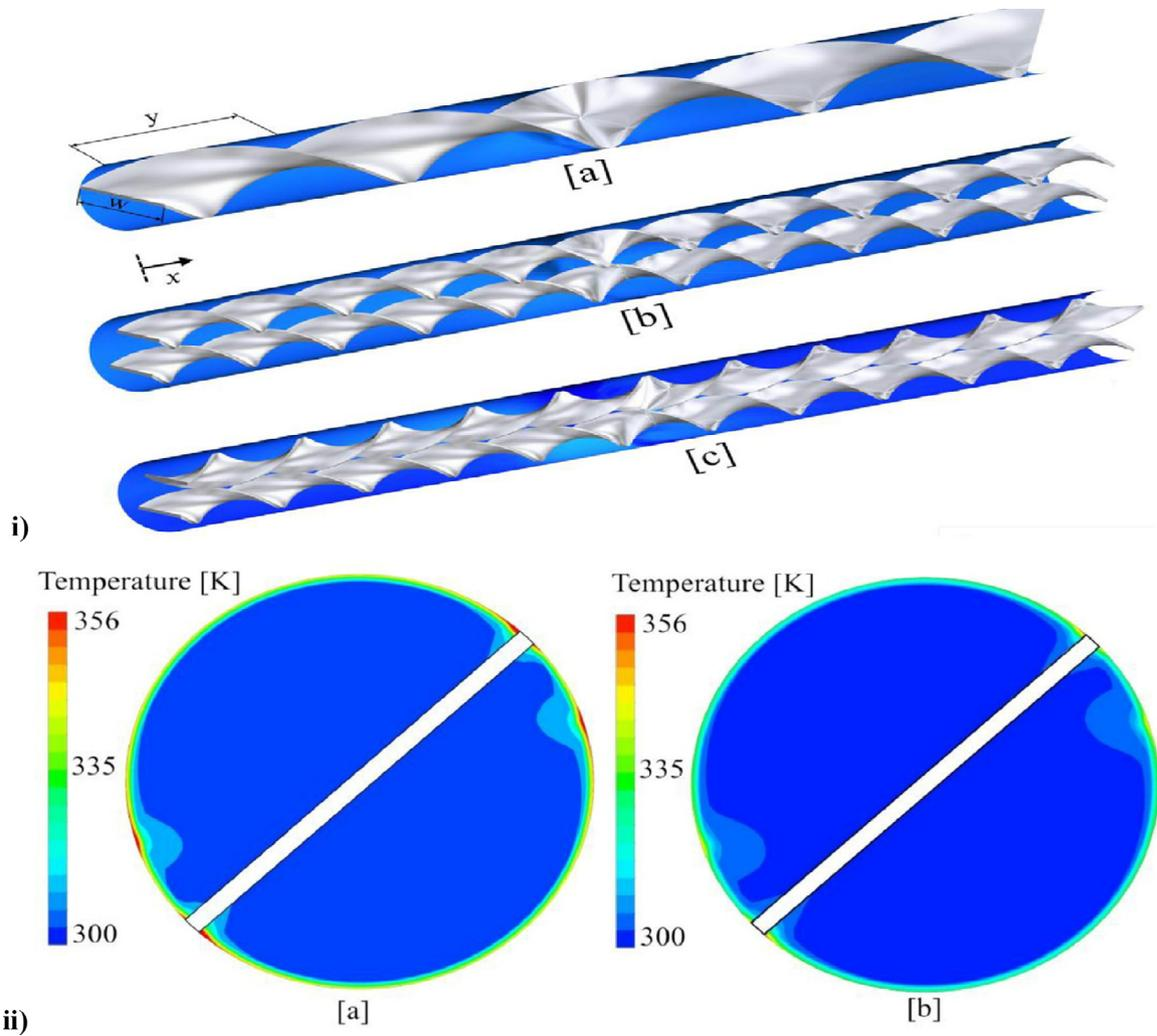
**Fig. 3.** (i) Geometry of the twisted tapes used for the investigation (a) Single twisted tape, (b) Co twisted tape, (c) Counter twisted tape; (ii) Temperature contours of single-twisted tape with twist ratio of 3 for: (a)  $\phi = 0\%$ , (b)  $\phi = 0.1\%$ , adapted with permission from Elsevier [51].
