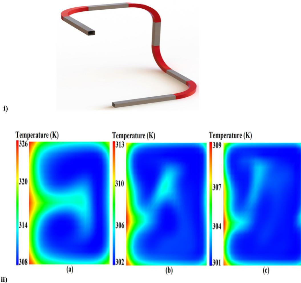
**Fig. 6.** (i) Chaotic geometry design studies, (ii) Temperature contours at Dean  $De$  number of (a) 100 (b) 300 (c) 500, adapted with permission from Elsevier [184].
