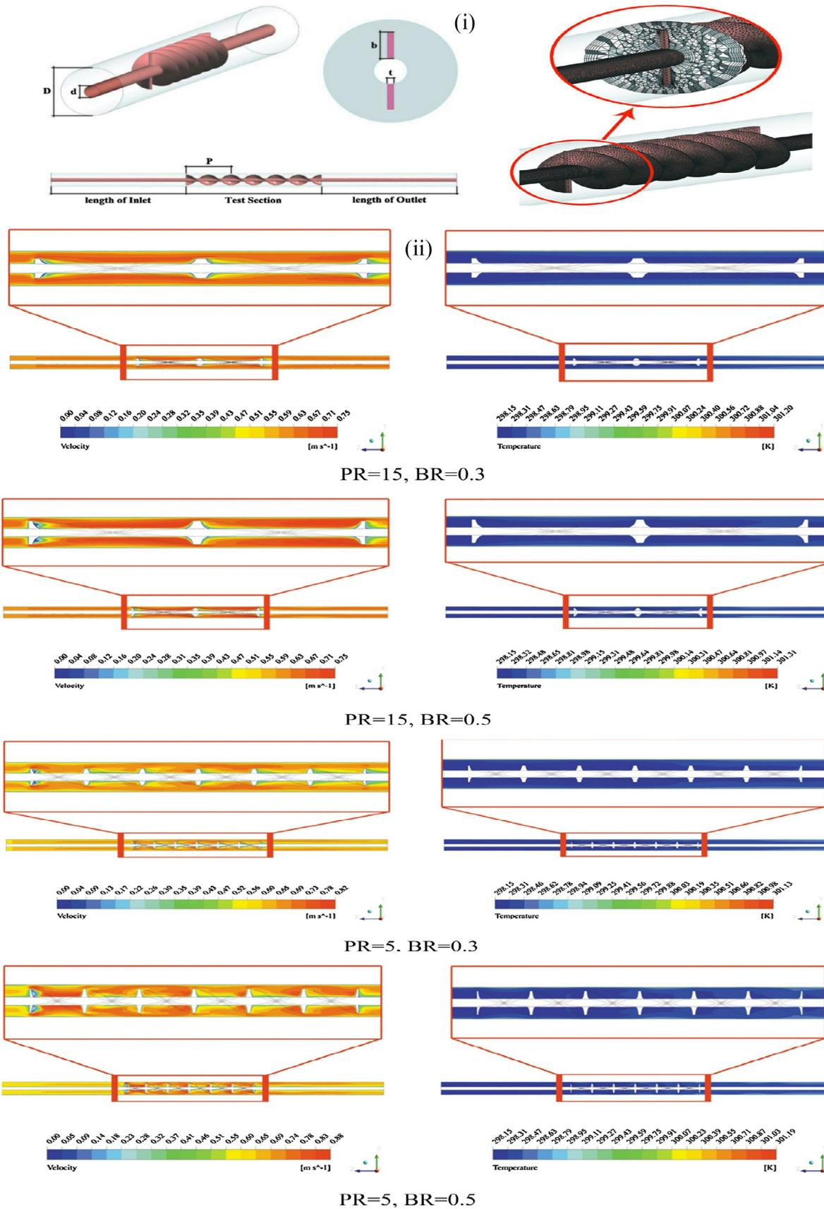
**Fig. 1.** (i) Geometry design and mesh used for circular cross-section, (ii) Velocity and temperature contours at  $Re$  of 2000 for different pitch and height ratios, adapted with permission from Elsevier [180].
