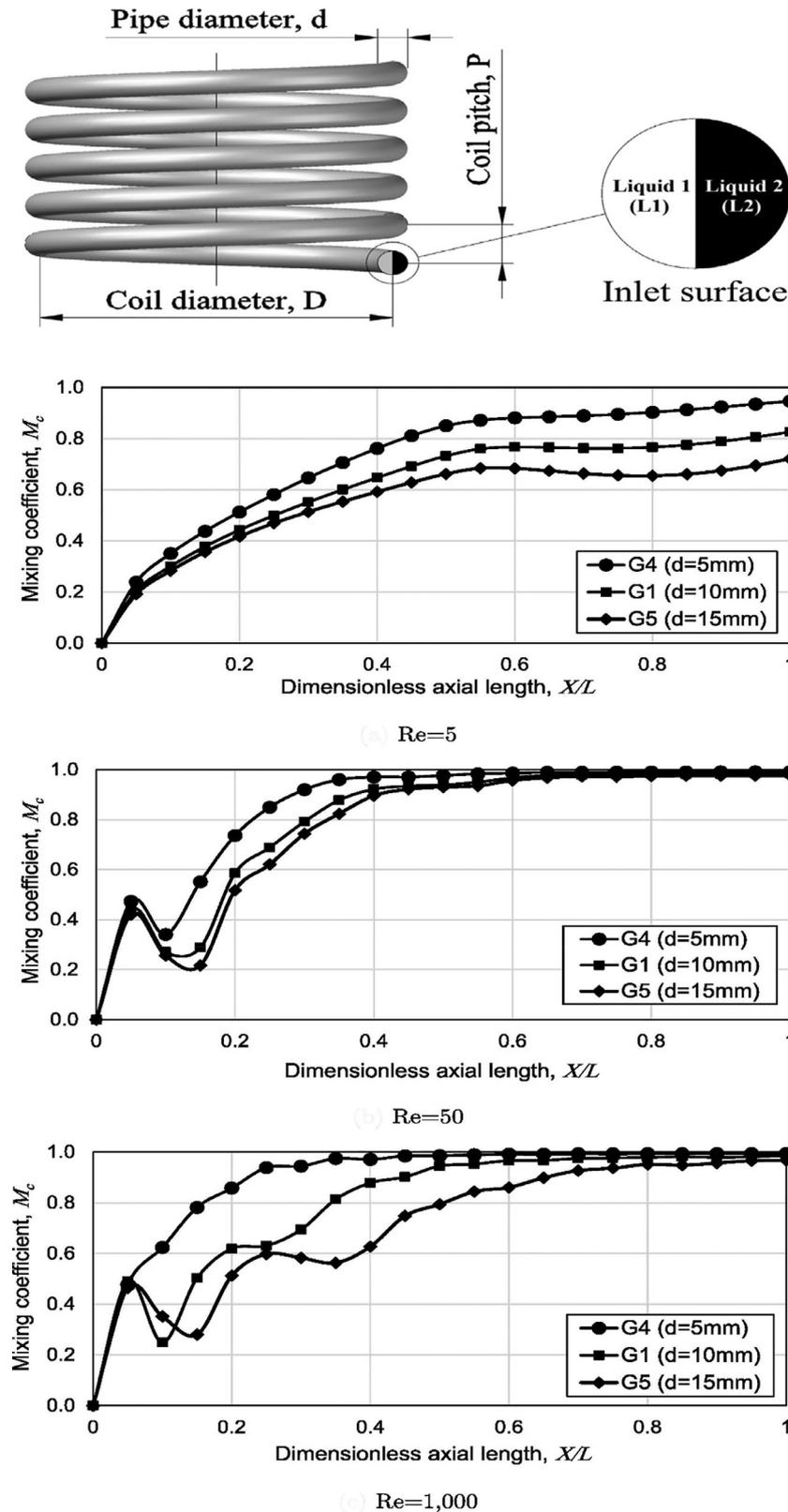
Fig. 5. Correlation between the pipe diameter and the mixing coefficient in the helical geometry pipe, adapted with permission from Elsevier [183].
