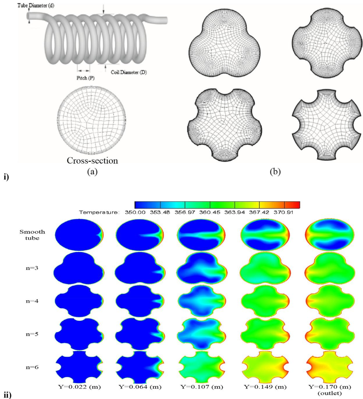
**Fig. 7.** (i) Geometry (a) Helical coil geometry design (b) Discretization carried out for the various geometry designs, (ii) Temperature contours of various cross-sections, adapted with permission from Elsevier [185].
