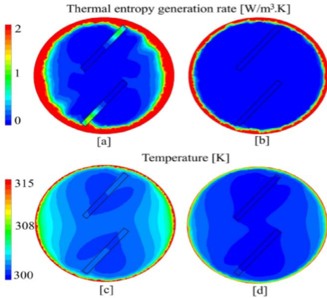
**Fig. 11.** Rate of thermal entropy generation for tube with co-twisted tapes [a] and [c] volume fraction  $\varphi = 0$ , [b] and [d]  $\varphi = 0.1$ , with permission from Elsevier [188].
