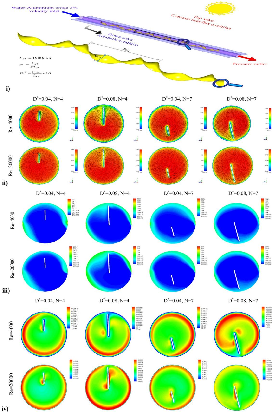
Fig. 15. (i) Geometry of the helical swirl, (ii) velocity contours, (iii) temperature contours, (iv) turbulence energy contours, adapted with permission from Elsevier [193].
