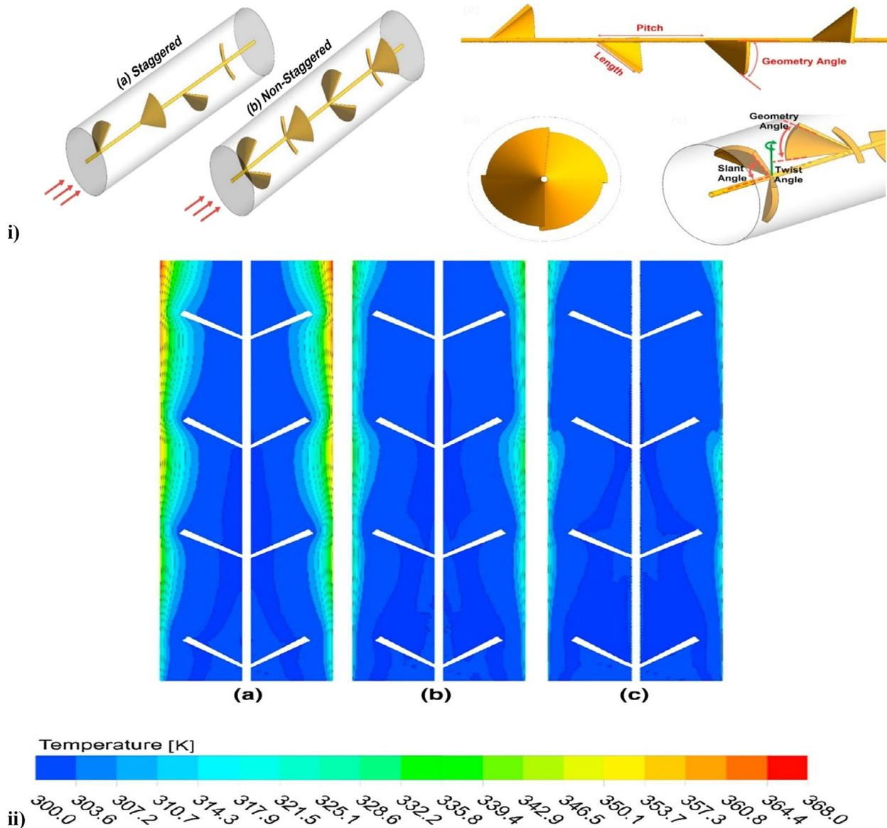
**Fig. 13.** (i) Geometry of twisted inserts, (ii) Temperature contours for non-staggered alignment at  $\phi = 3\%$  for: (a)  $Re = 100$ , (b)  $Re = 300$ , and (c)  $Re = 700$ , adapted with permission from Elsevier [75].
