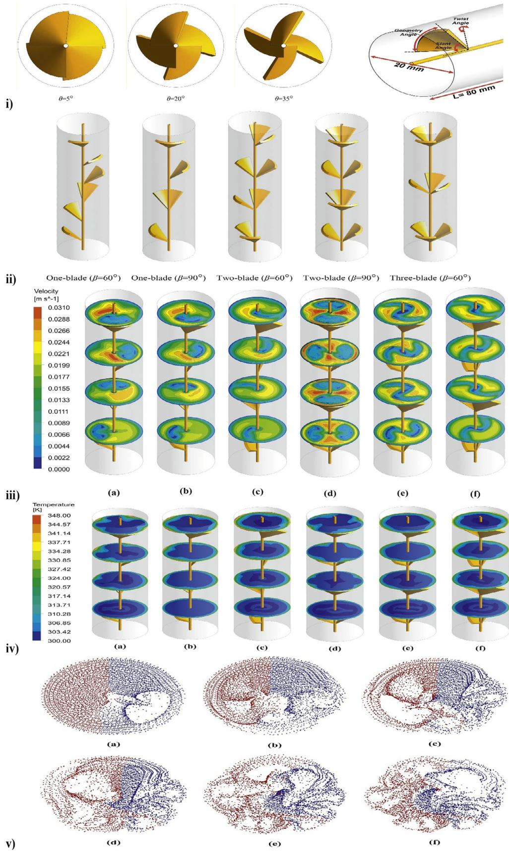
**Fig. 9.** (i) and (ii) geometry, (iii) velocity contours, (iv) temperature countours, (v) particles dispersion for various twist configurations: (a)1B,  $\theta = 5^\circ$ , (b) 1B,  $\theta = 20^\circ$ , (c)1B,  $\theta = 35^\circ$ , (d) 2B,  $\theta = 5^\circ$ , (e) 2B,  $\theta = 20^\circ$ , (f) 2B,  $\theta = 35^\circ$ , adapted with permission from Elsevier [187].
