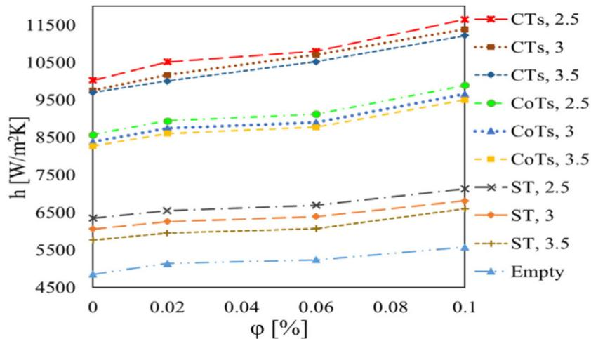
**Fig. 4.** Convective heat transfer coefficient for the single twisted (ST), twin co-twisted (CoTs), and counter twisted (CTs) tape configurations at different twist ratios, with permission from Elsevier [51].
