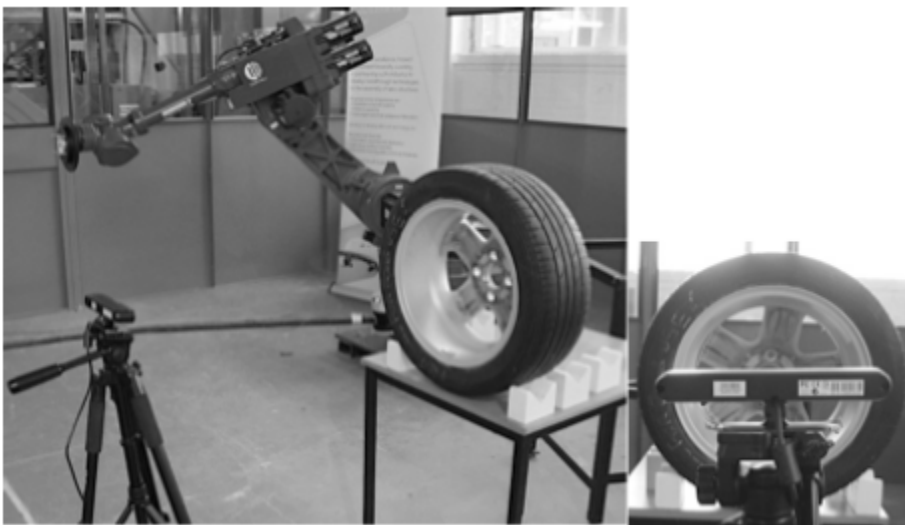
Fig. 4 Data capture of Wheel parameters using Xtion (Prabhu et al., 2014).
