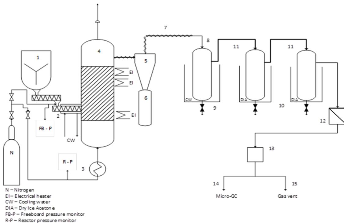
Figure 1. Bench scale 300 g h<sup>-1</sup> fluidised bed fast pyrolysis rig set-up.
