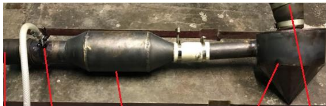
Inlet Injection point Expansion pipe Swirl chamber Outlet
