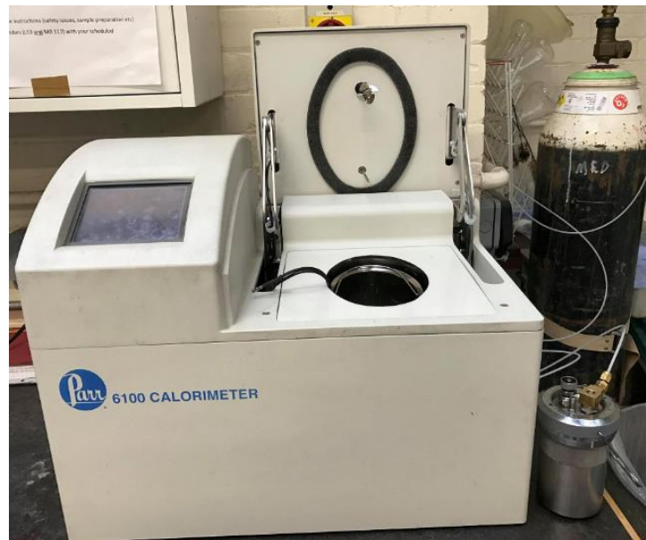
Figure 3.9: Parr 6100 calorimeter used for Higher Heating Value measurement (Aston University mechanical engineering laboratory).
