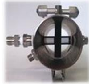
Figure 3.21: Tailpipe attachment, sampling part with water trap.
