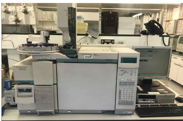
Figure 3.12: Gas Chromatography and mass spectrum equipment used to quantify FAME, TAG, DAG and MAG (Aston University, European Bioenergy Research Institute).
