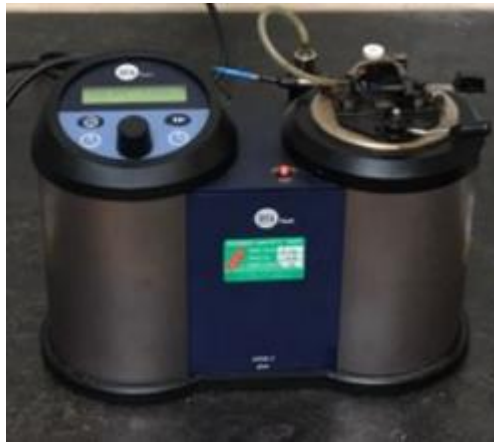
Figure 3.8: Flash points of biodiesels were measured through Setaflash Series 3 Closed Cup flash point tester (Aston University mechanical engineering laboratory).
