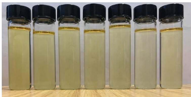
Figure 4.3: Biomixtures obtained by blending waste cooking oil biodiesel (W100) and sheep fat biodiesel (A100); from left to right W100, W80A20, W60A40, W50A50, W30A70, W10A90 and A100.
