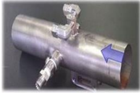
Figure 3.21: Tailpipe attachment, sampling part with water trap.
