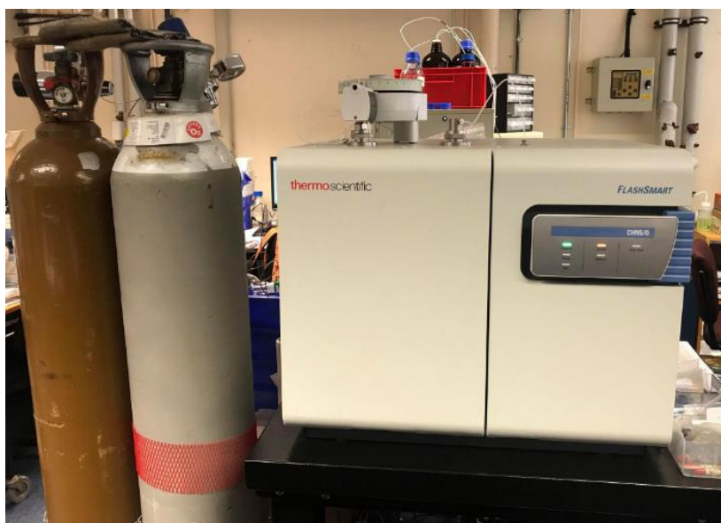
Figure 3.10: Elemental analyser equipment used to measure carbon, hydrogen and nitrogen contents of biodiesels and biomixtures (University of Birmingham).
