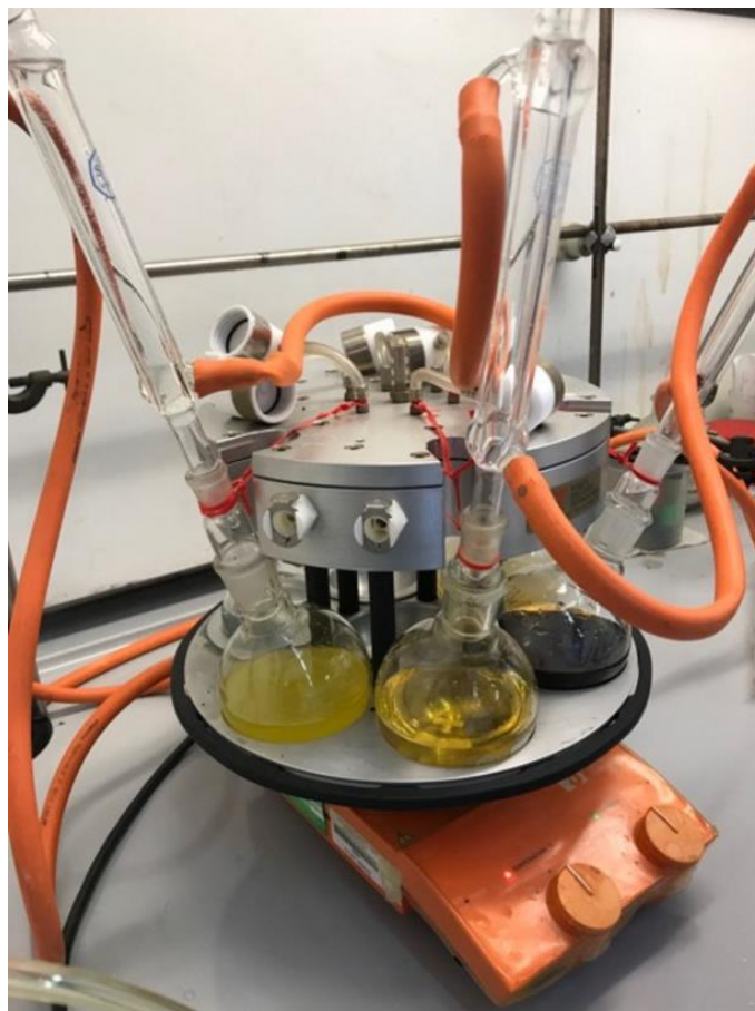
Figure 3.3: Transesterification setup which includes heating from the bottom, continuous mechanical string with a help of magnets and condenser at the top (Aston University chemistry laboratories).
