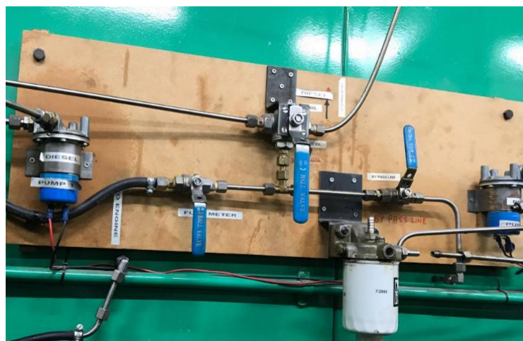
Figure 3.16: T-junction placed on the dual fuel supply system.
