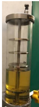
Figure 3.19: Graduated cylinder installed on fuel supply system to measure fuel consumption.
