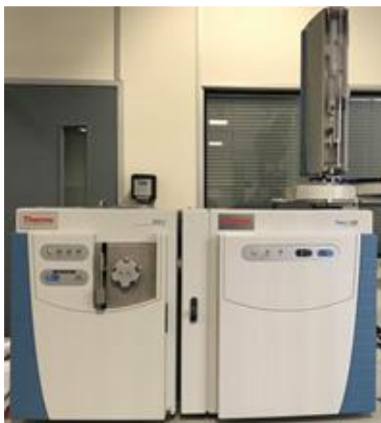
Figure 3.11: Gas Chromatography and mass spectrum equipment used to determine FAME compositions (Aston University, chemical engineering laboratory).
