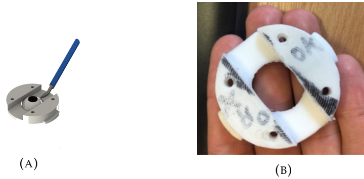
FIGURE 6.5: Modified perfusion chamber allowing greater tissue exposure to the surgeon while practicing cataract surgery. (A) represents the 3D CAD rendering, while (B) shows the 30mm groove manufactured in PTFE.
