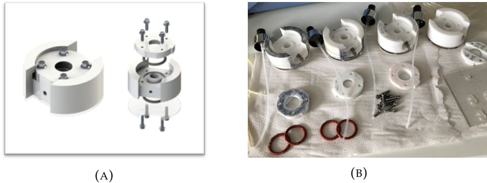
FIGURE 5.5: Perfusion module design and manufacturing. SOLIDWORKS renderings (A) and final prototypes manufactured in PTFE (B).
