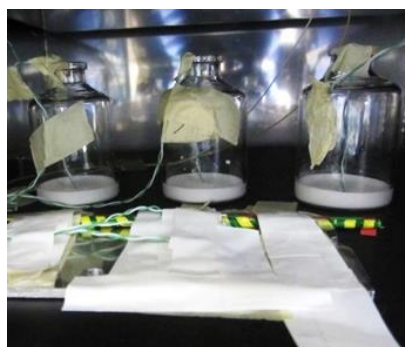
Figure 114 POFBG sensor positioned on the shelf next to 3 vials containing 5ml 10%w/v mannitol. K-type thermocouples were inserted into the centre of the vial to monitor product temperature during freeze drying
