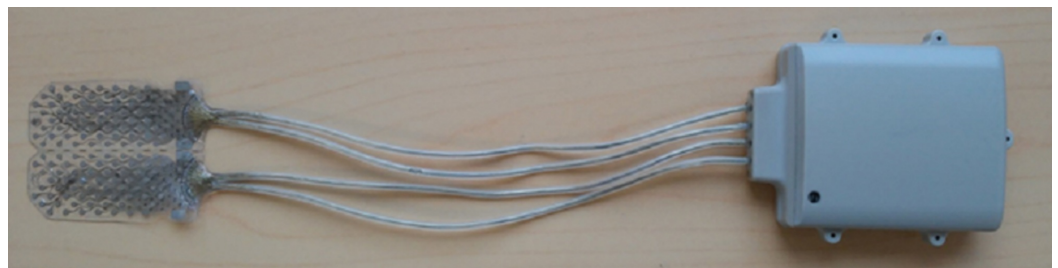
FIGURE 1: ECoGI-64D - the picture shows the subdural grid, connecting cables and a wireless case
