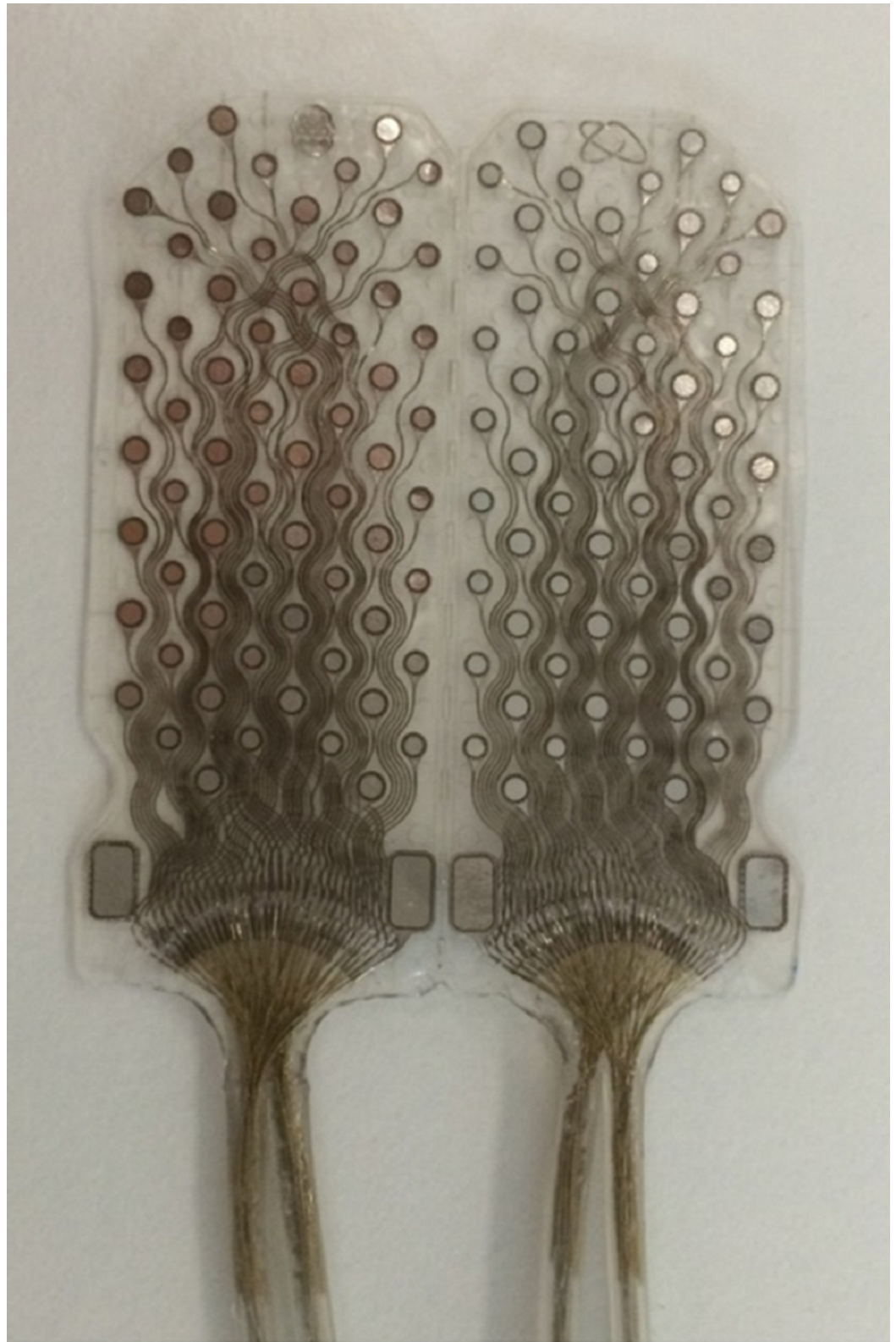
FIGURE 2: The 128 contacts subdural grid hosting 64 recording and 64 stimulating contacts plus four ground contacts
