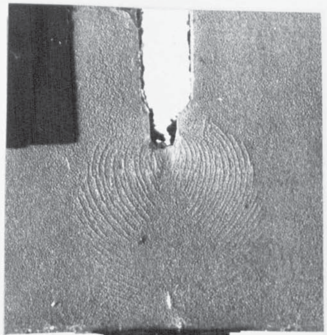
D X 3.6 \rho = 1.5 mm. Specimen NO. 16 Photo taken when test stopped at P = 2.24 tones.
