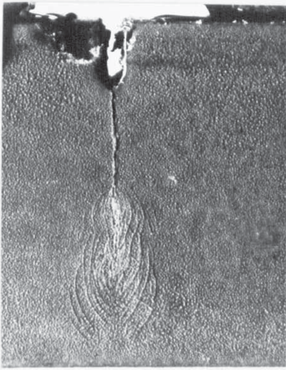
A X3.6 \rho = 0.127 mm. Specimen NO. 11 Photo taken when test stopped at P = 1.22 tones.
