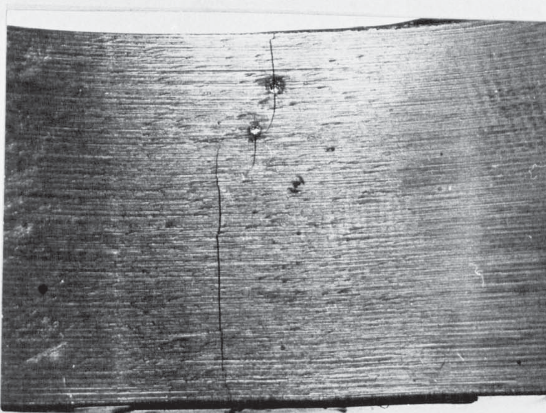
Figure 51a Several macro-cracks for a 25.4 mm notch root radius specimen
