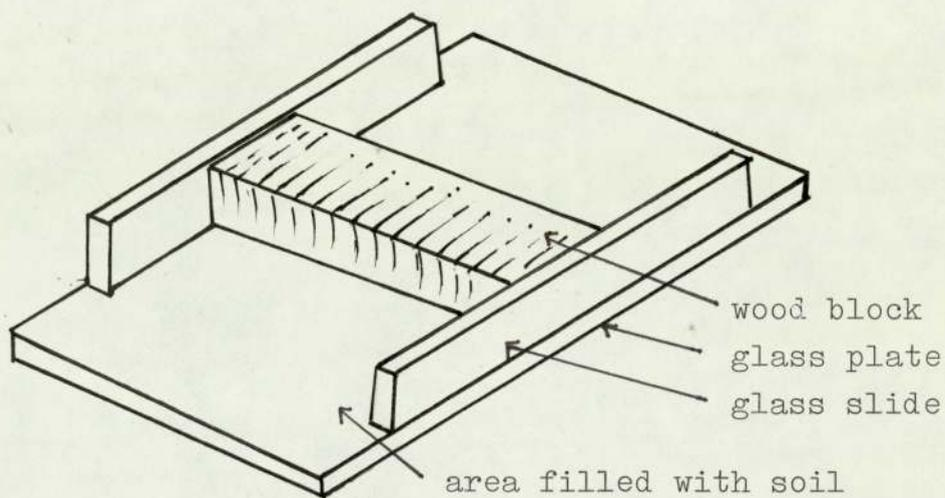
Fig.7. Diagram showing arrangement of wood block and soil on glass plate used for studying the effect of soluble nutrients in wood on the activity of soil microorganisms.
