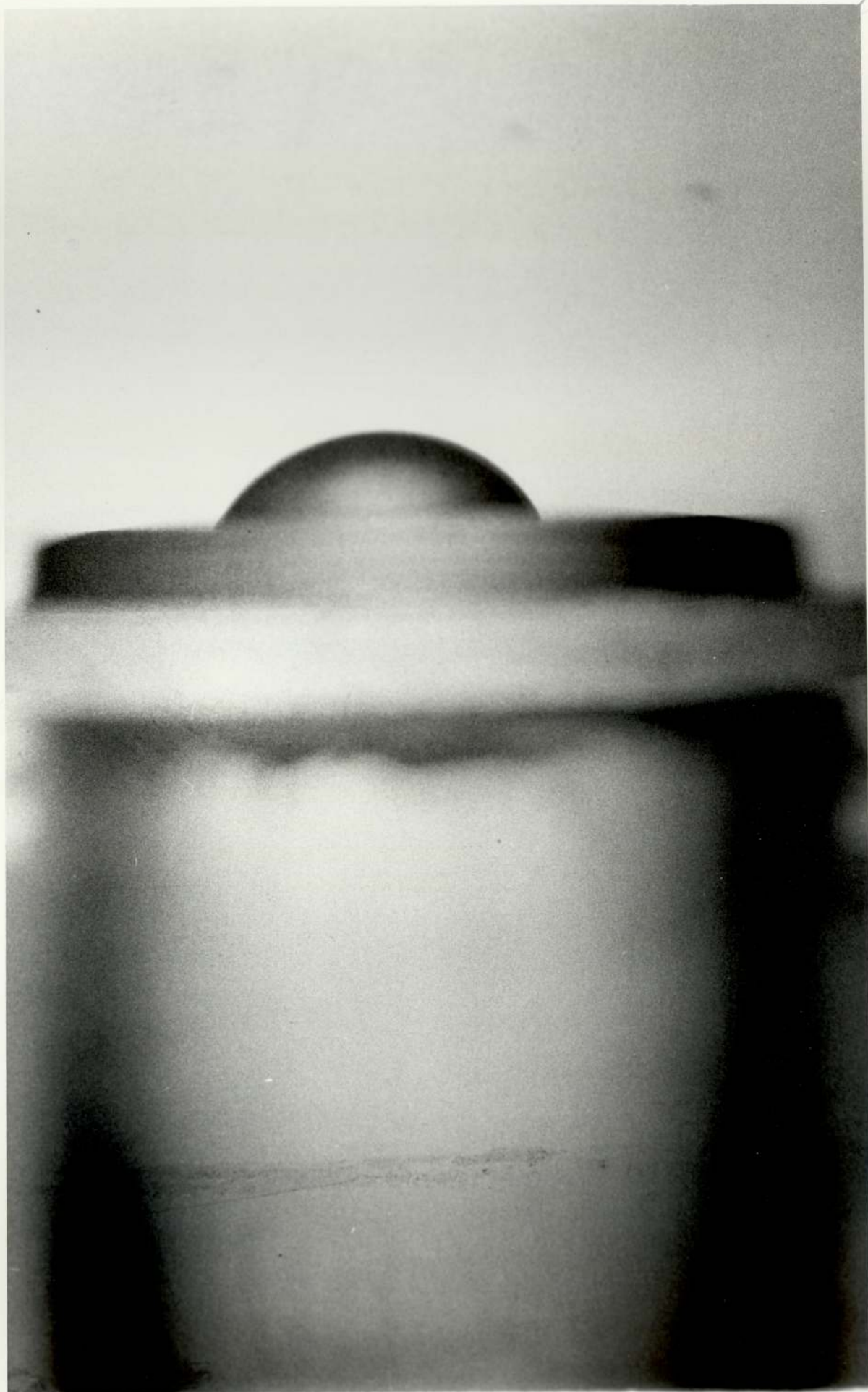
PLATE 3 Projected Image of Water Droplet on Polymer Disc
