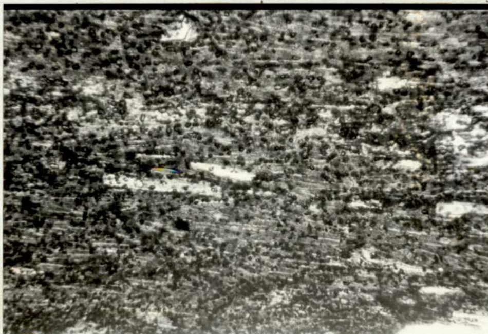
Plate 5B. Effect of increasing flow rate showing increase in filler orientation, Phenolic PF 17A, (PF 17B similar)
