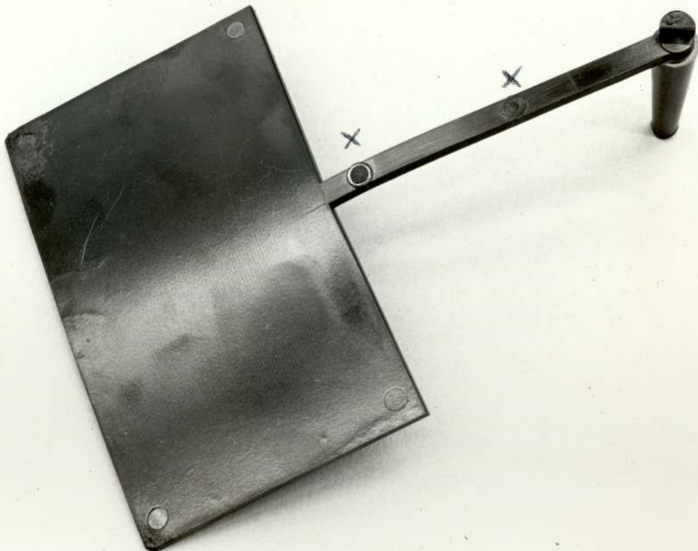
Plate 8. Moulding from runner viscometer/plaque mould.
