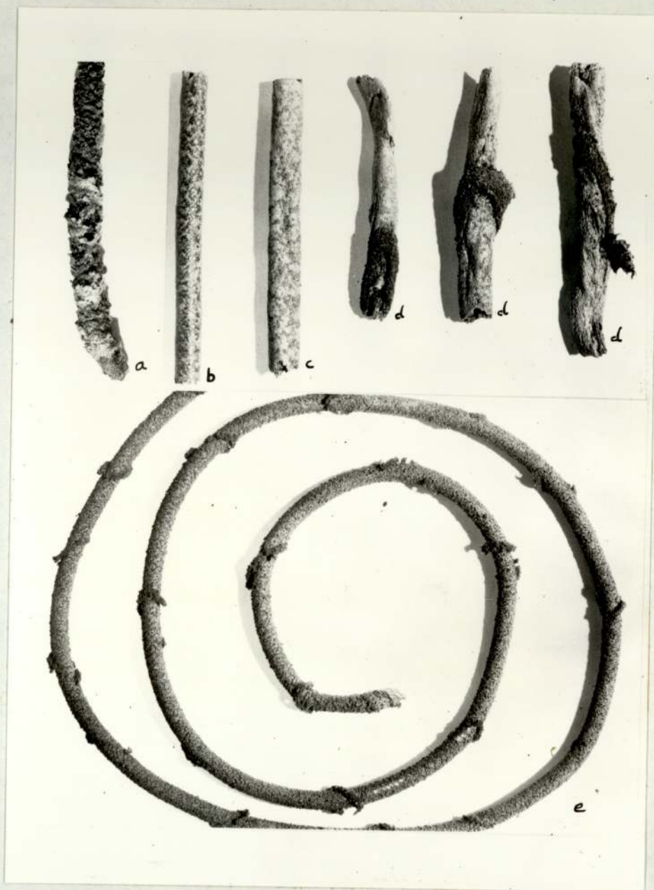
Plate 4. Effect of increasing flow rate on the surface of the extrudate. Phenolic PF 17A.
