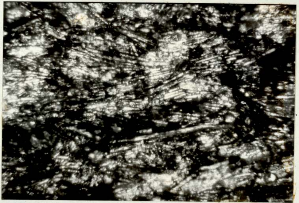
Plate 6A. Effect of increasing flow rate showing increase in filler orientation, Melamine MF 24E.
