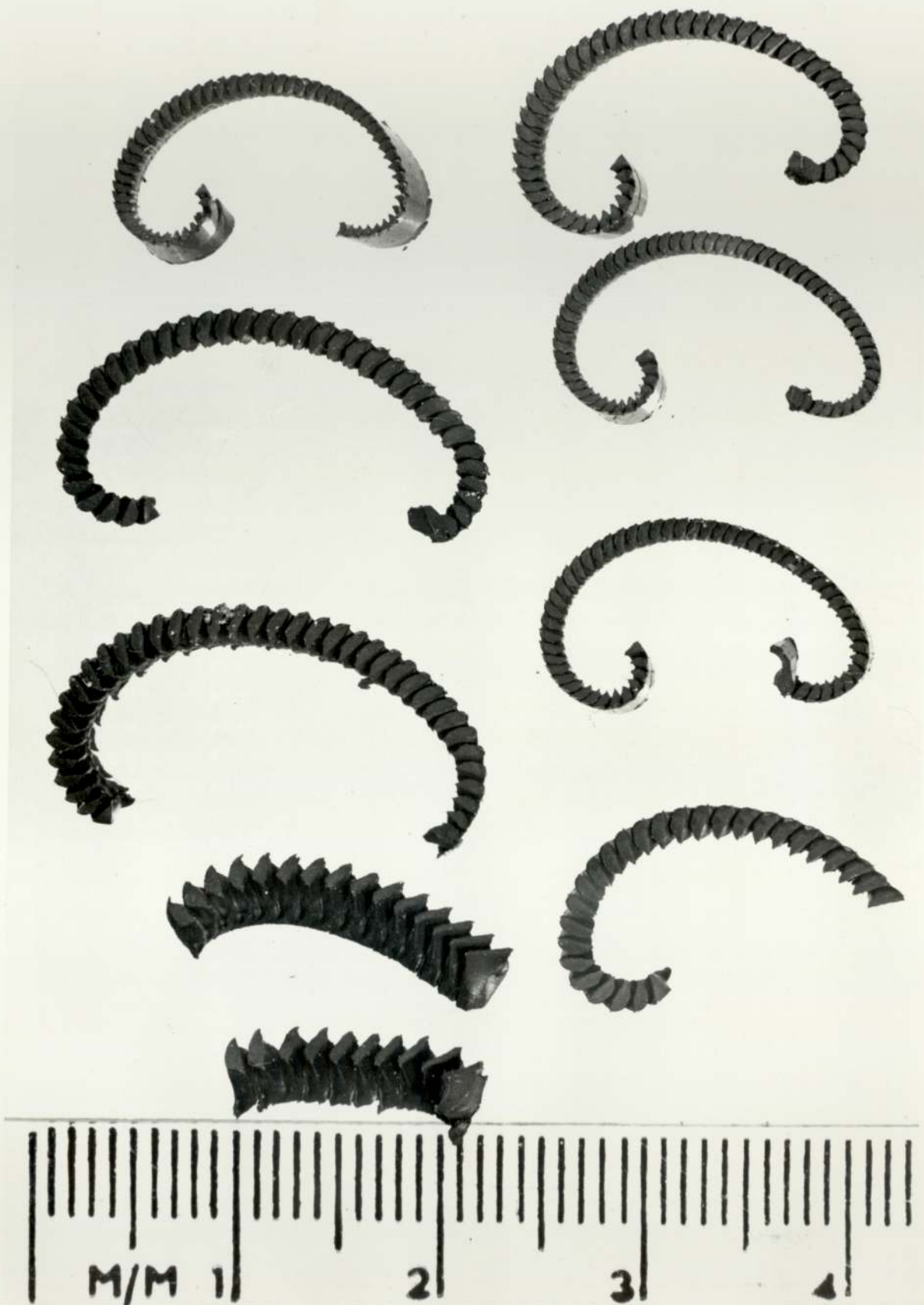
Fig.22 Chips Obtained under the Conditions of Cutting Speed of 182.21 m/min, F 1.666 m/min, d 2.03 mm, W 57 mm
