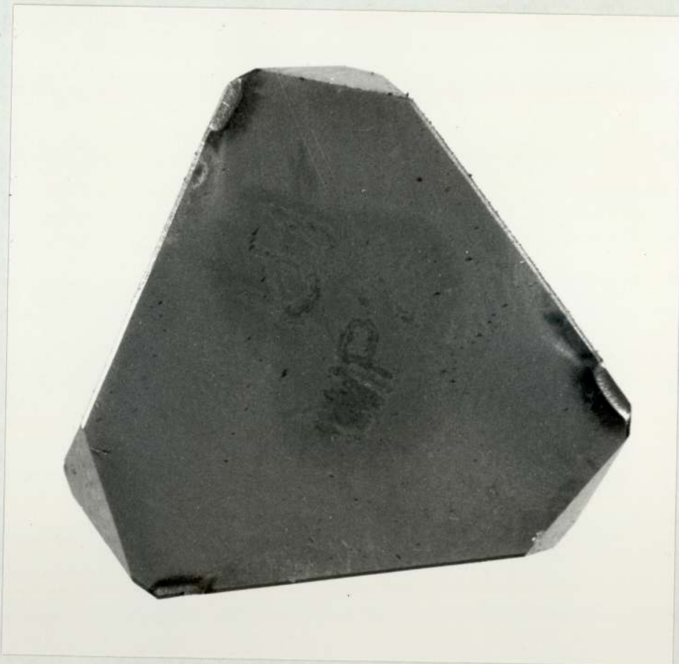
Fig.23 Crater Wear on One Insert using with the Sandvik Cutter
