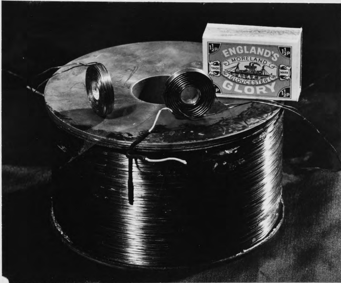
Figure 3.4 Two miniature lens windings supported by the conventional winding they replace.
