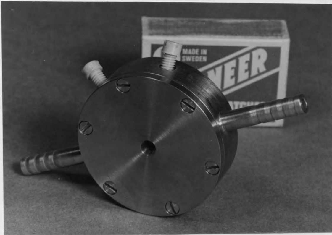
Figure 6.3 Assembled 2000 A-t projector lens. The nylon terminals provide water tight seals for the coil leads. Length of matchbox is 50 mm.
