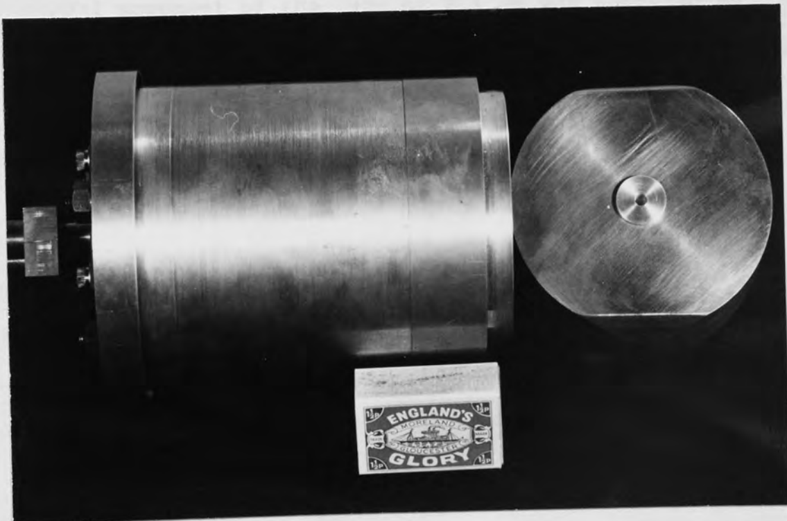
Figure 10.11 The million volt lens, viewed from above showing the duralumin X-ray limiting aperture (18.6 mm dia.), in the lens bore. Notice the flats machined on the lens surface to allow entry of the lens into the porthole.
