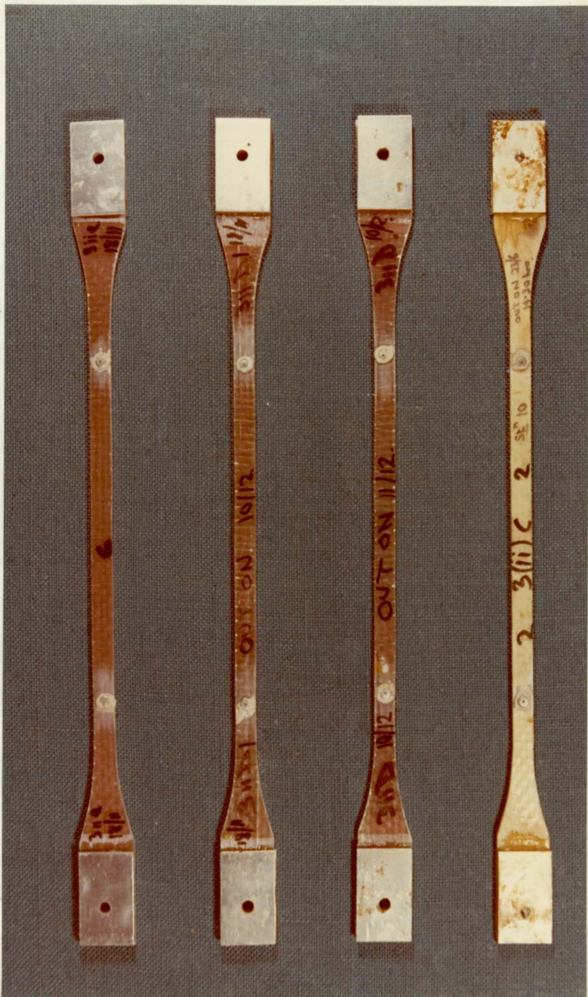
FIG. 3.33 CREEP SPECIMENS - UNIDIRECTIONAL
