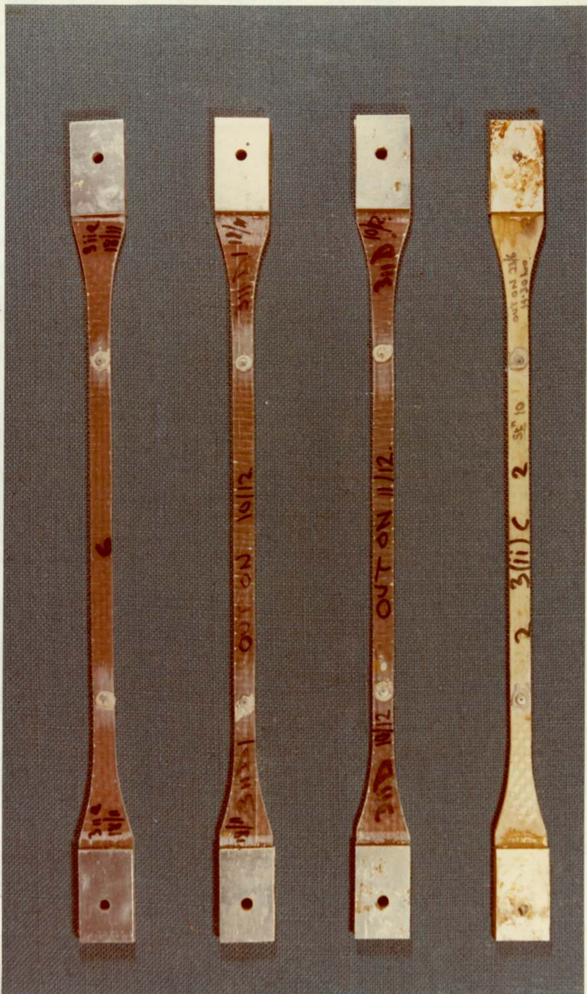
FIG. 3.33 CREEP SPECIMENS - UNIDIRECTIONAL
