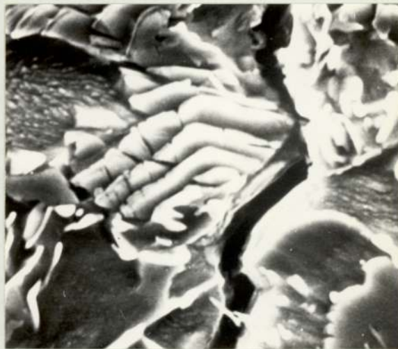
Plate 40. Material L Crack Propagation Path. Scanning Electron Micrograph. ( x 8.2k ).
