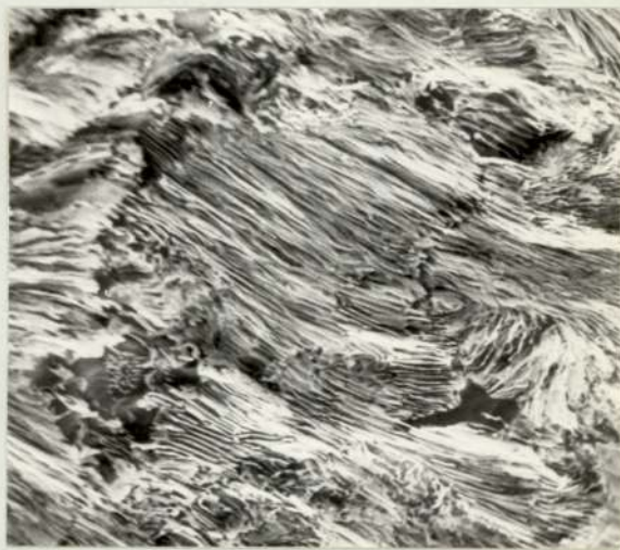
Plate 62. Material L Fast Fracture Surface electro-etched. Scanning Electron Micrograph. ( x 1200 ).
