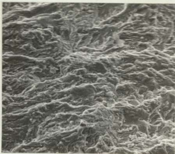
Plate 64. Material B Fatigue Fracture Surface. Scanning Electron Micrograph. ( x 600 ).
