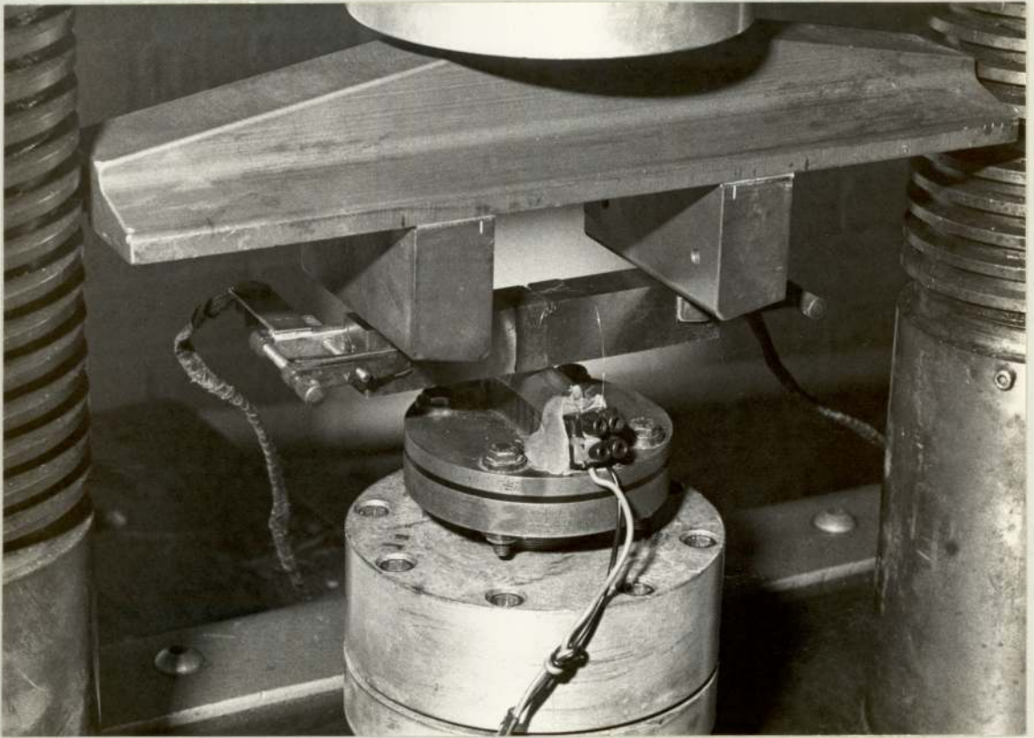
Plate 3. Specimen Located in the testing rig with current leads and potential probes attached.
