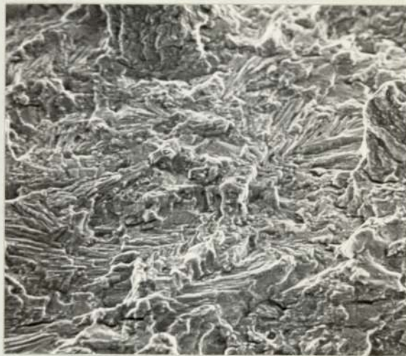
Plate 58. Material A Fracture Surface at Intermediate Growth Rates. Scanning Electron Micrograph. ( x 950 ).
