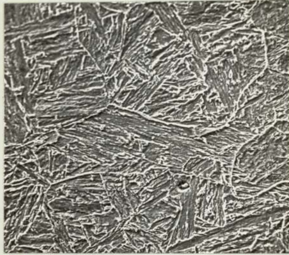
Plate 21. Material G Microstructure. Scanning Electron Micrograph. ( x 750 ).
