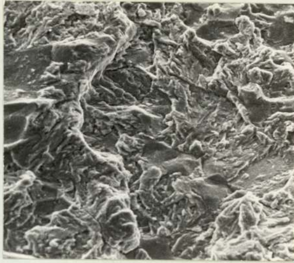
Plate 67. Material C Fatigue Fracture Surface. Scanning Electron Micrograph. ( x 600 ).
