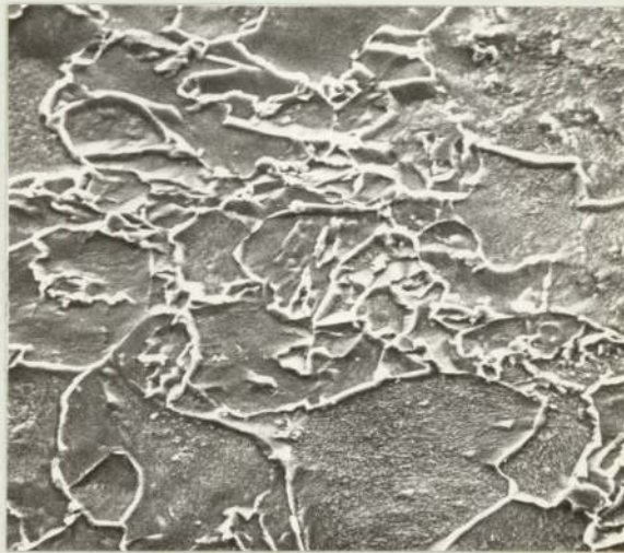
Plate 15. Material BT Microstructure. Scanning Electron Micrograph. ( x 400 ).
