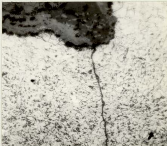
Plate 88. Material G Crack Initiation at a Surface Imperfection. Optical Micrograph. ( x 500 ).
