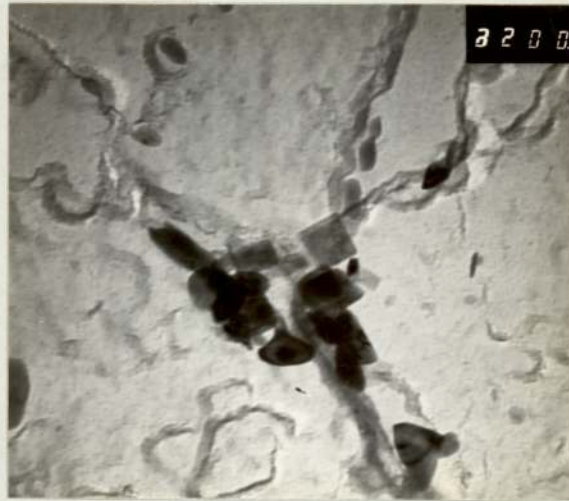
Plate 18. As Plate 16. Triple point carbide segregation. ( x 200k ).
