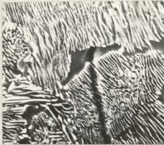
Plate 44. Material L Crack Tip. Scanning Electron Micrograph. ( x 2100 ).
