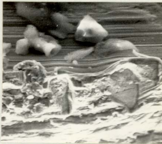
Plate 82. Material G Notch Surface Debris. Scanning Electron Micrograph. ( x 1800 ).
