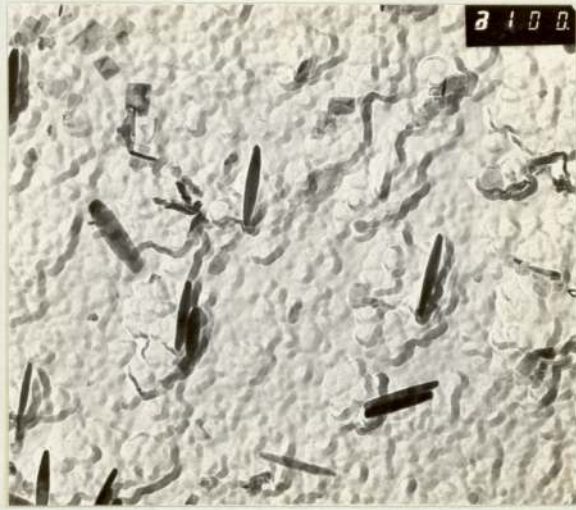
Plate 19. Material BT Extraction Replica. Transmission Electron Micrograph. ( x 100k ).
