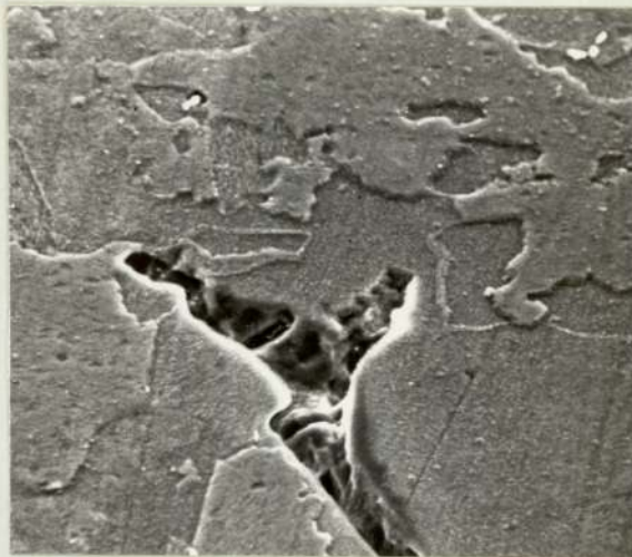
Plate 48. Material B Crack Tip. Scanning Electron Micrograph. ( x 10k ).
