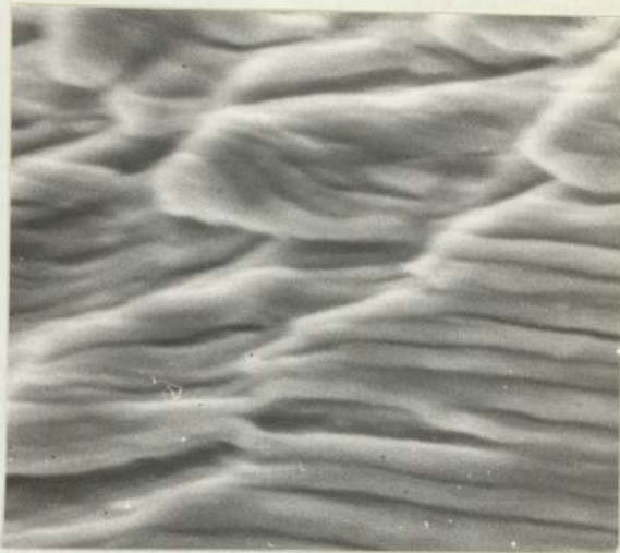
Plate 81. OFHC Copper Fatigue Striations. Scanning Electron Micrograph. ( x 2000 ).
