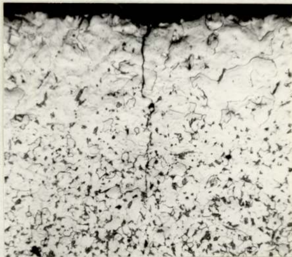
Plate 84. Material B Cast Specimen Microstructure. Optical Micrograph. ( x 100 ).
