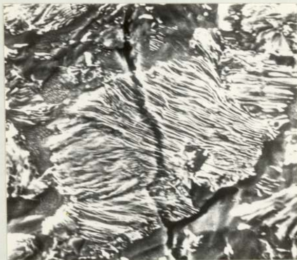
Plate 42. Material L Unfractured Cementite Plates. Scanning Electron Micrograph. ( x 1250 ).
