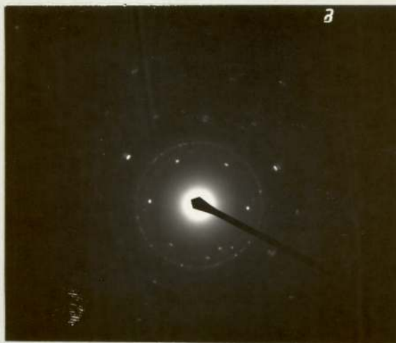
Plate 18a. Diffraction Pattern of an Extracted carbide.
