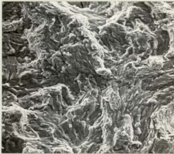
Plate 56. Material A Fracture Surface close to the Notch root. Scanning Electron Micrograph. ( x 1100 ).
