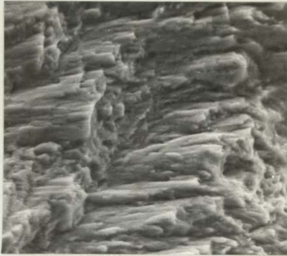
Plate 69. Material F Inter-plate Separation. Scanning Electron Micrograph. ( x 1200 ).
