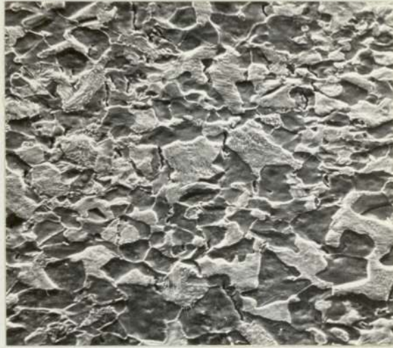
Plate 25. Material A Crack Initiation Sites. Scanning Electron Micrograph. ( x 500 ).
