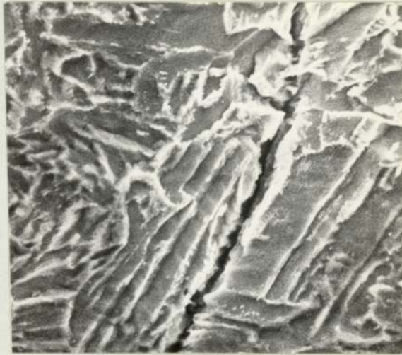
Plate 49. Material F Crack Propagation Path. Scanning Electron Micrograph. ( x 2200 ).
