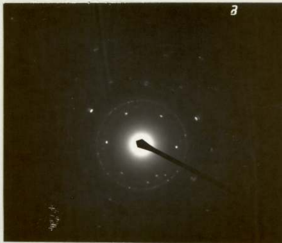
Plate 18a. Diffraction Pattern of an Extracted carbide.
