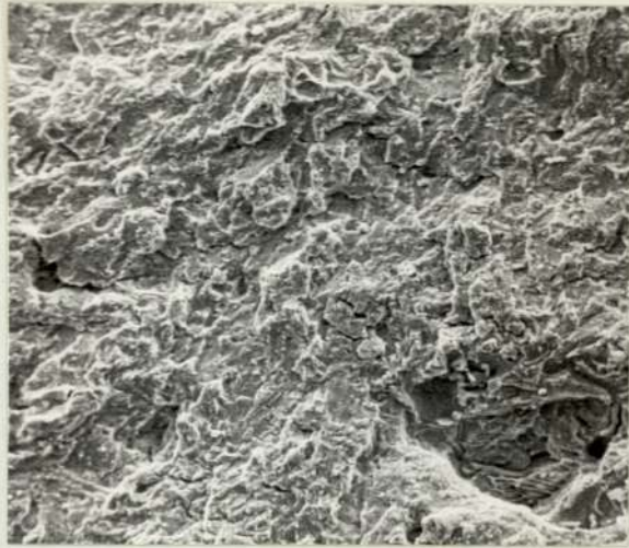
Plate 57. Material A Fracture Surface at Fast Fracture. Scanning Electron Micrograph. ( x 750 ).
