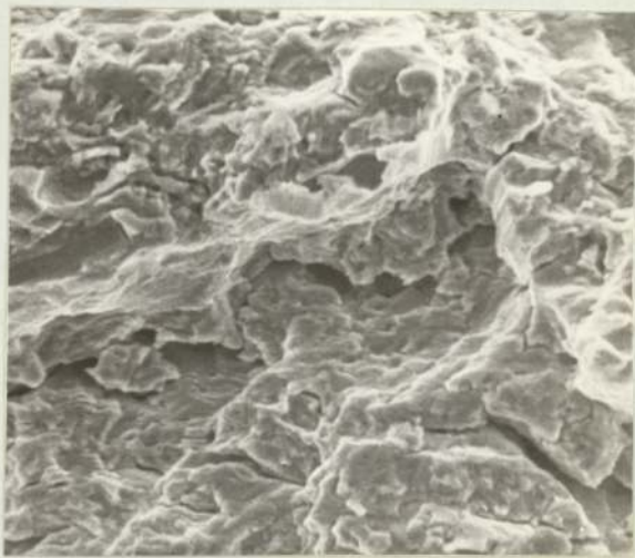
Plate 60. Material A Secondary Cracking. Scanning Electron Micrograph. ( x 1500 ).
