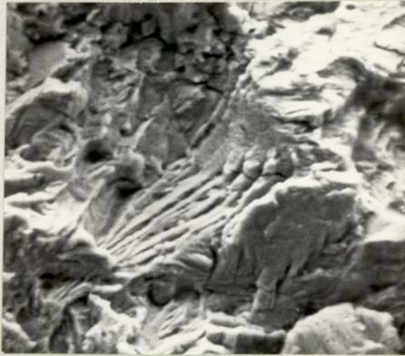
Plate 59. Material A Pseudo-striations. Scanning Electron Micrograph. ( x 1800 ).
