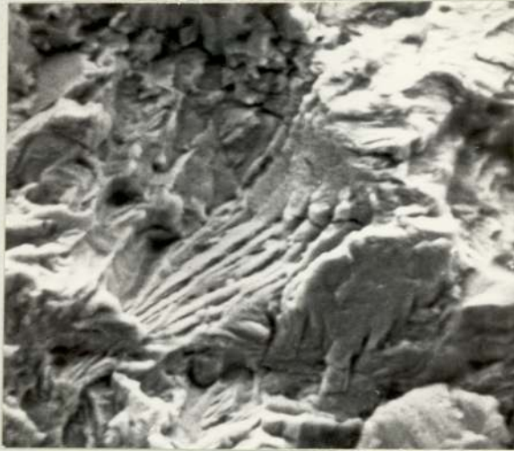
Plate 59. Material A Pseudo-striations. Scanning Electron Micrograph. ( x 1800 ).
