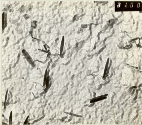
Plate 19. Material BT Extraction Replica. Transmission Electron Micrograph. ( x 100k ).
