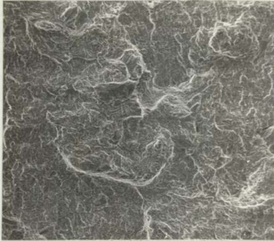
Plate 71. Material F Fast Fracture Surface. Scanning Electron Micrograph. ( x 550 ).
