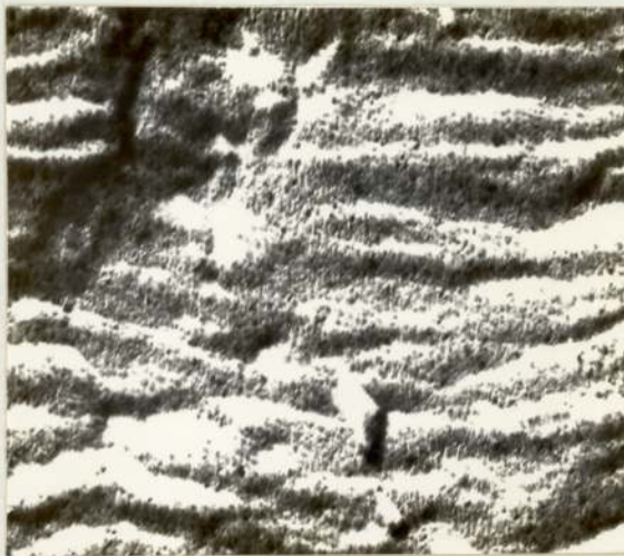
Plate 80. Material G Striation Formation. Transmission Electron Micrograph. ( x 50k ).
