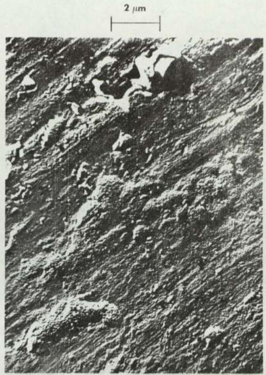
(b) Wear track on the plate at 100 C
