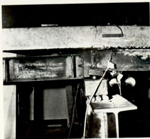
Plate 7. Lever arm connection at the support to the secondary beam.
