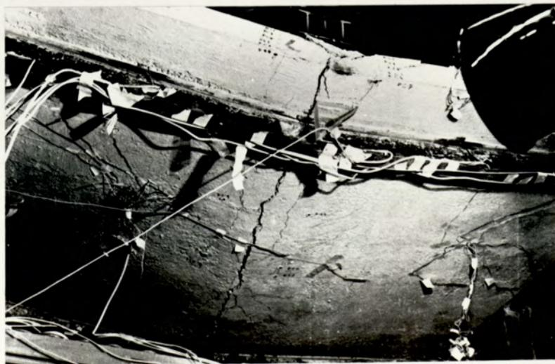
Plate 20. Formation of plastic composite hinges at mid-span of model  $M_3$  after control test  $C_1$ .
