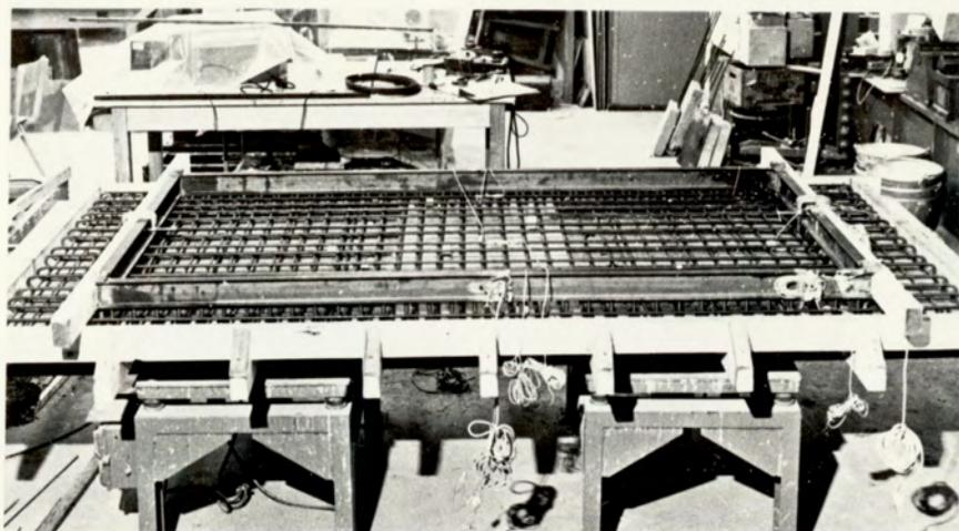
Plate 4. Model before casting.
