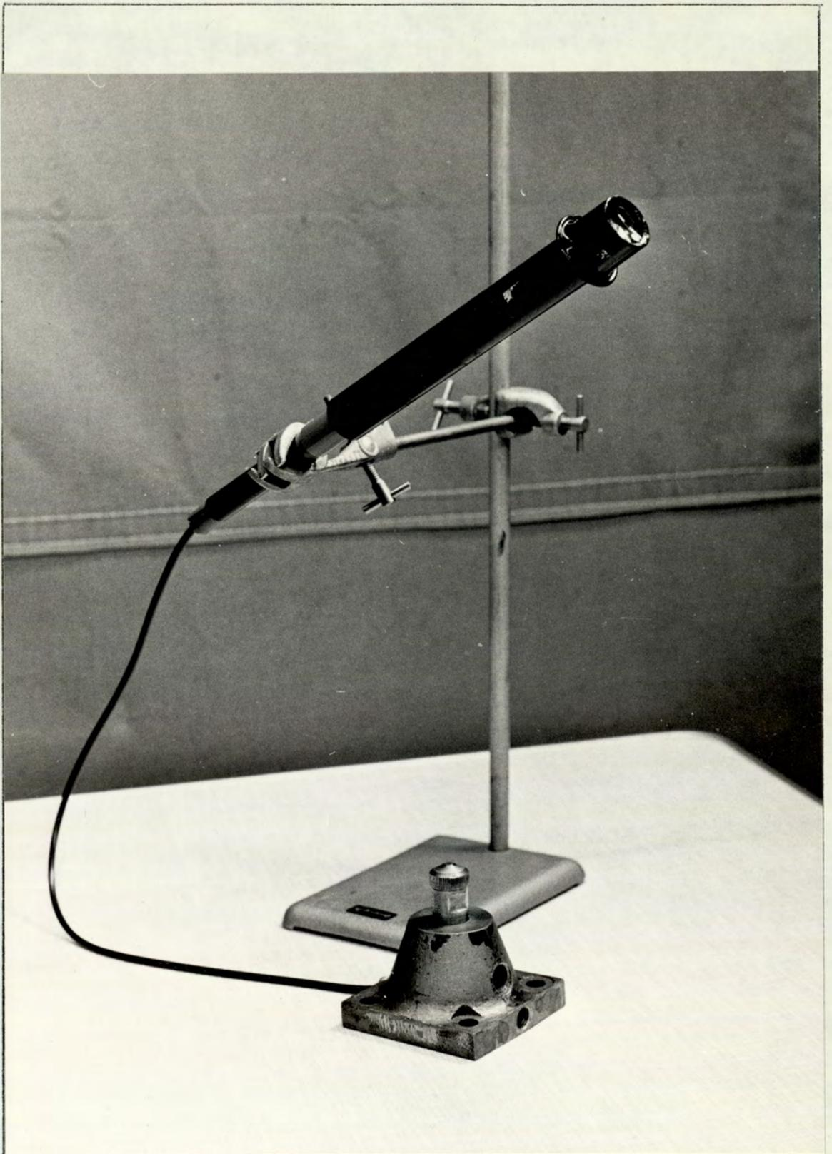
FIG. 10.3. Apparatus for Visual Observation of Weld Glow
