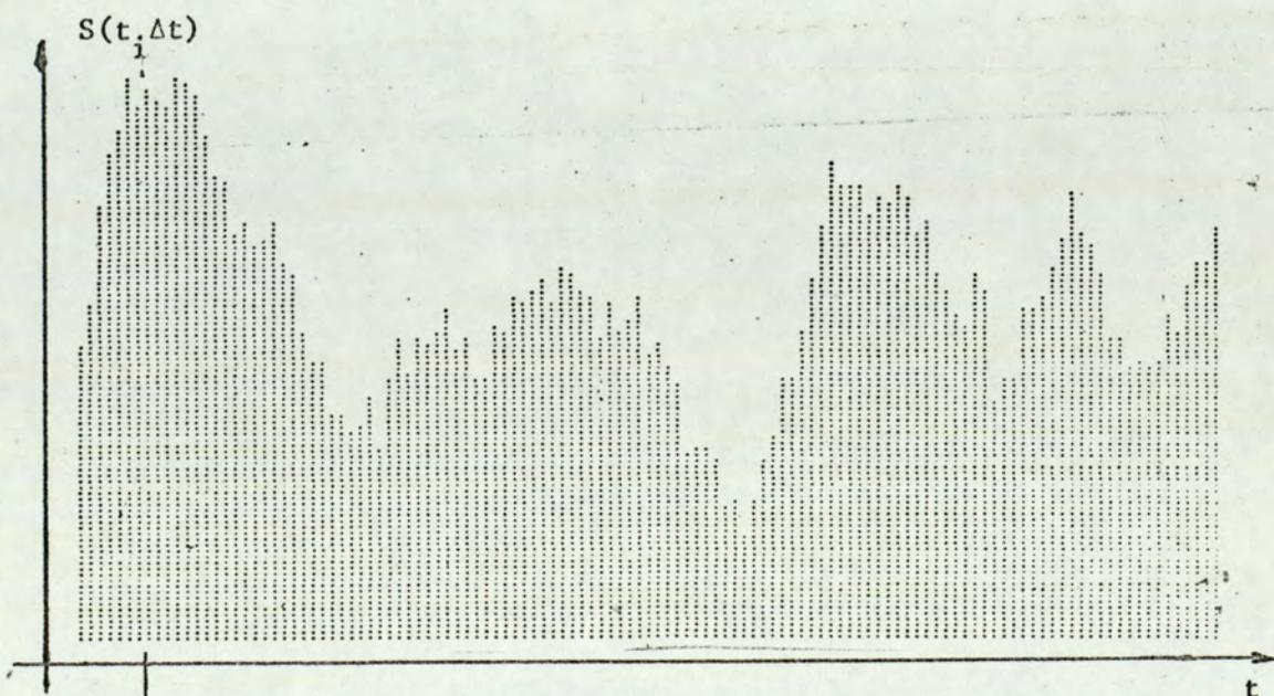
Fig.2.1 An actual signal magnitude fluctuation obtained in an experiment made for this research ( $\Delta t_s = 4\text{msec}$ ). (No phase lock).
