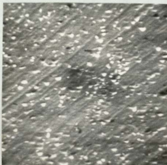
Fig. 9.4.1. Stereoscan photographs of cementite precipitated as a consequence of overaging after a standard annealing treatment; a) overaged at 300^{\circ}\text{C} for 1 hour, b) overaged at 200^{\circ}\text{C} for 5 hours c) overaged at 150^{\circ}\text{C} for 25 hours. Mag X 12500
